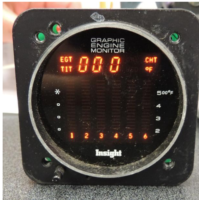
Figure 1. Photo of GEM-603 with power applied.
