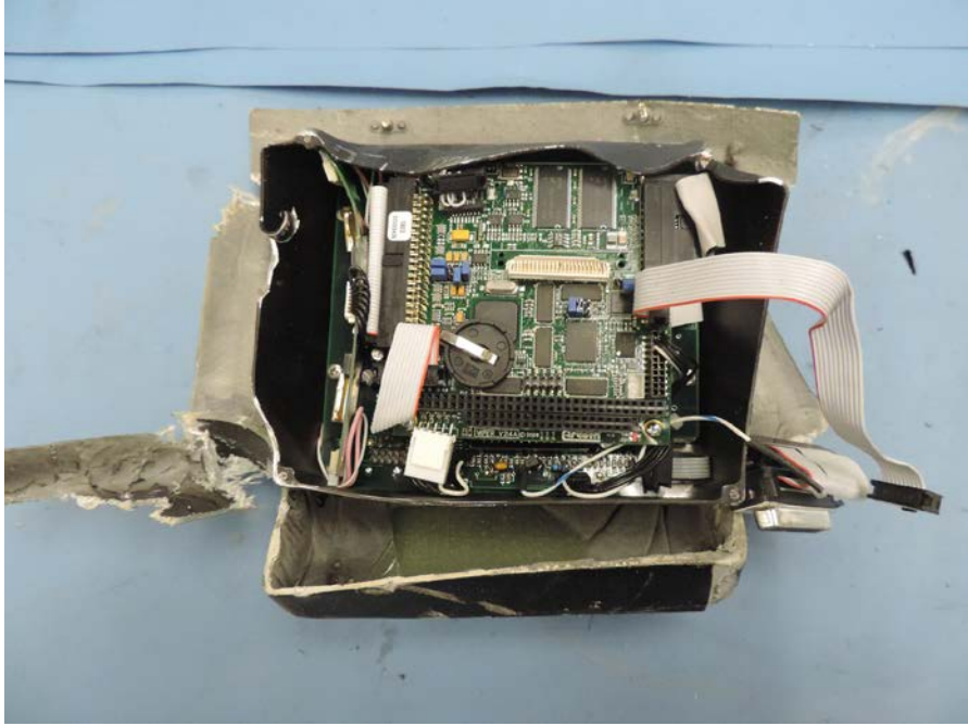
Figure 1. MVP-50 as received with back of housing missing.
