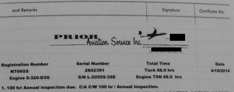
2. Hot cylinder compression check due. C/A C/W Hot compression check # 1 75/80, # 2 78/80, # 3 76/80 and # 4 74/80.
