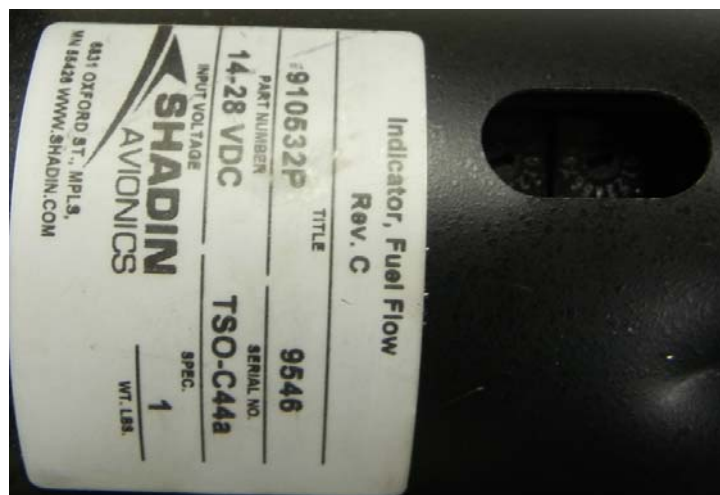
Figure 2. Shadin Digiflo-L™ side of unit, and cut-out for switch settings.
