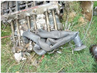
Induction System Condition: The induction system exhibited impact damage. All six induction risers exhibited impact damage. The induction manifold was fractured free of the engine and located in the debris field.
