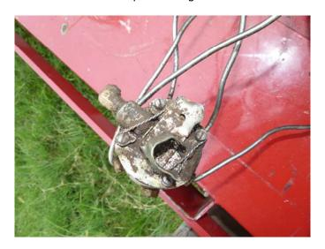
Throttle Body / Metering Unit Manufacturer: TCM Part Number: 652844-1A4 Serial #: A06FA034
