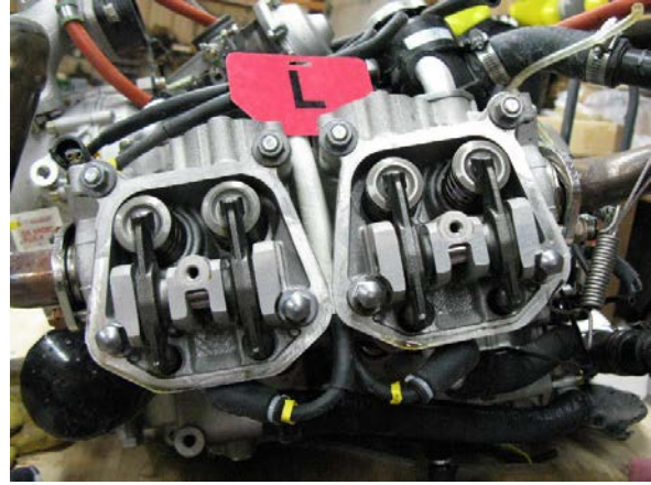
Photo 4: Rocker Arm and Valve Assembly – Cyl. 2 & 4
