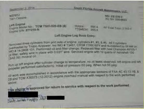
**NOTE:** The total time on this engine at this maintenance event was 1763.50 hours. The hobbs meter was replaced with zero-time unit 9-12-2002 with instructions to add 868.1 to hobbs for actual left engine time since factory rebuilt.
