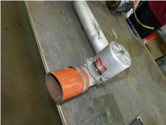
Over Boost Valve: Kelly, PN-470944-12, SN-HF0251 The over boost valve was not damaged.
