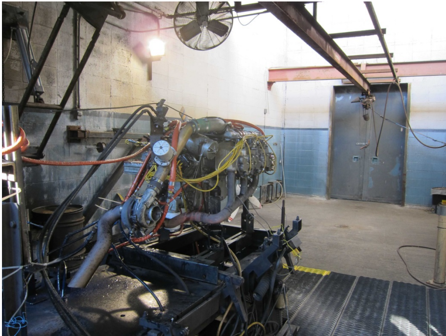
Photo 11 - Front Engine Operating In Test Cell
