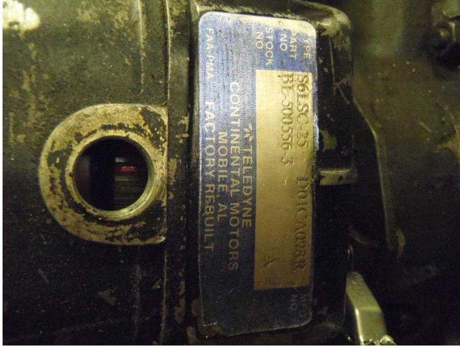
Photo 8 - Front Engine - Right Magneto Timing Inspection Hole
