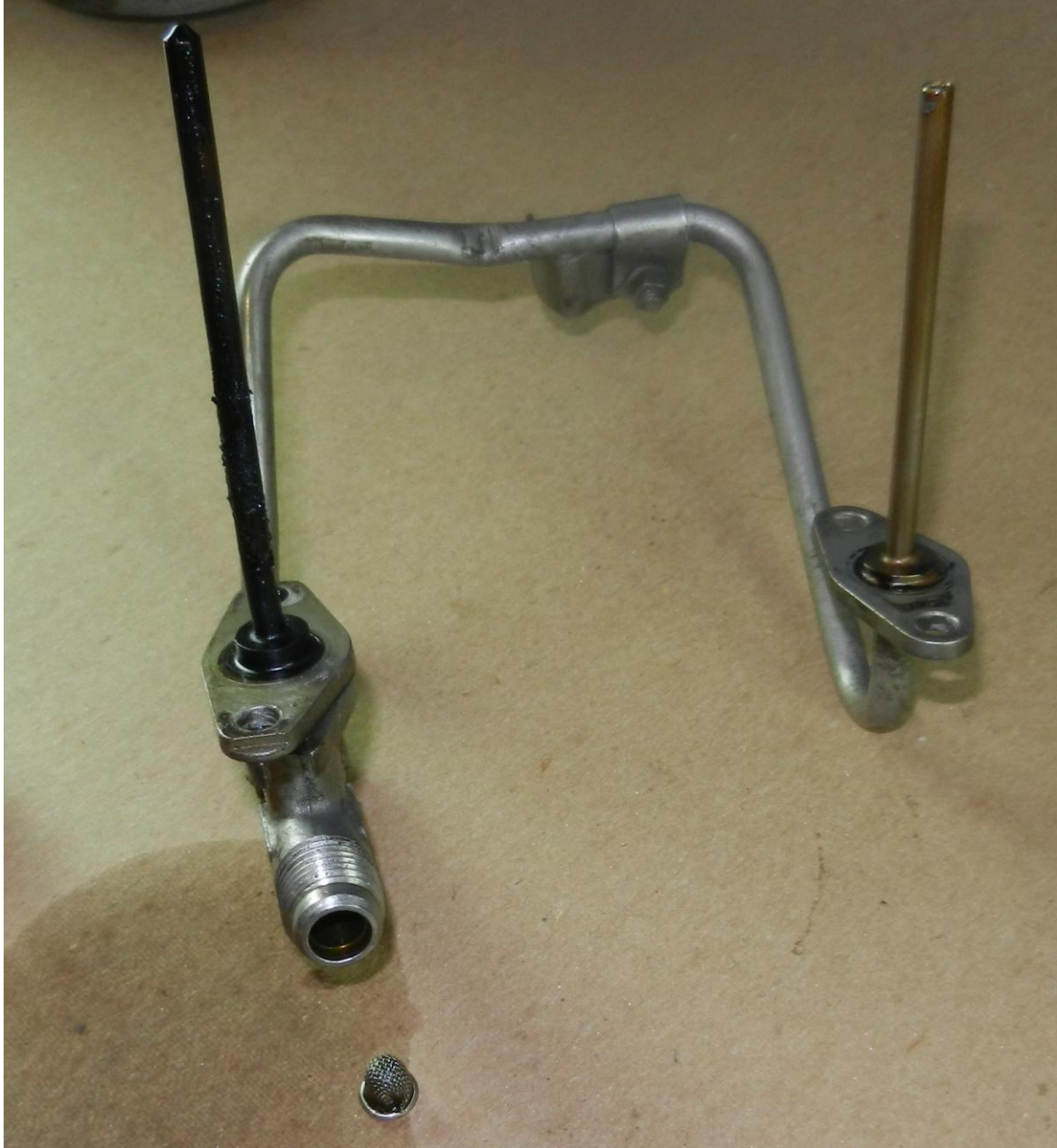
No. 6 and 7 Bearing Oil Pressure Tube, Oil Pressure Screen, and No. 8 Oil Pressure Tube
