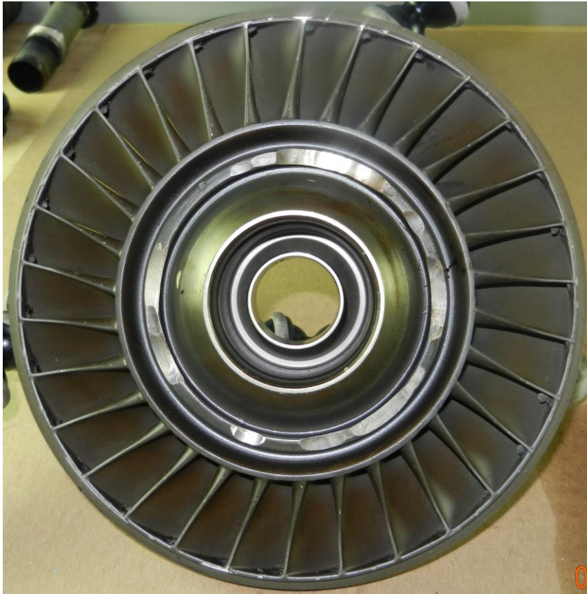
Fig: 14 3 rd Stage Turbine Wheel and Nozzle
