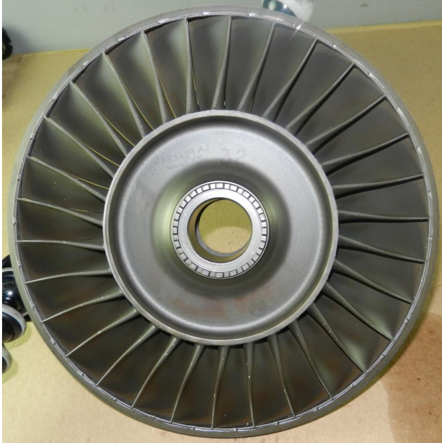
Fig: 15 4 th Stage Turbine Wheel and Nozzle
