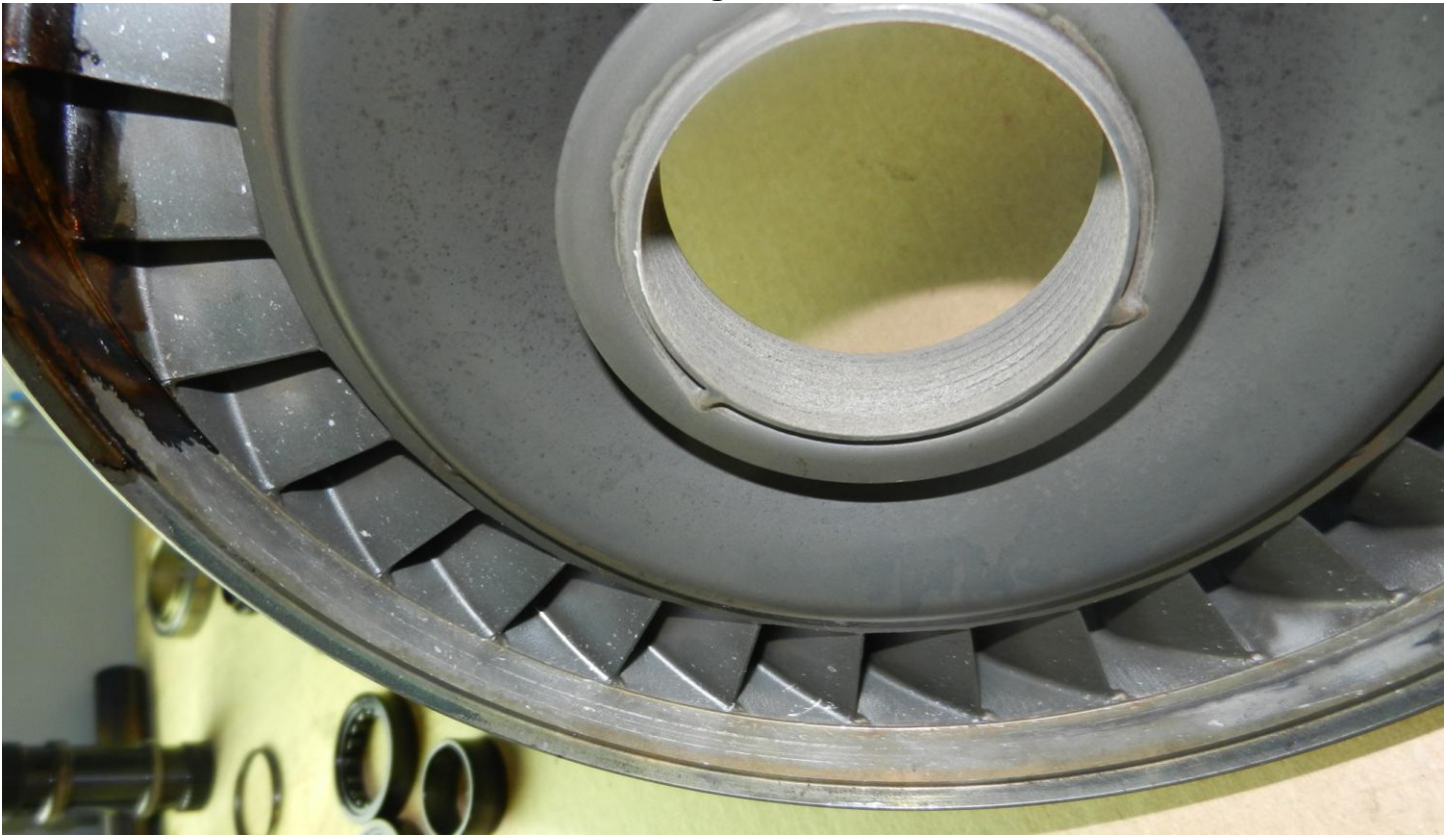
2 nd Stage Turbine Wheel Blade Tracks
