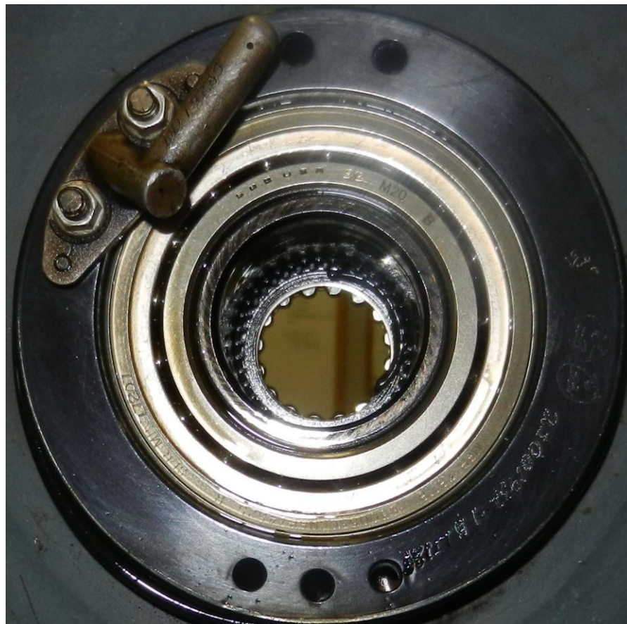
No. 2 ½, 3, and 4 Bearing As Viewed Through the Gearbox
