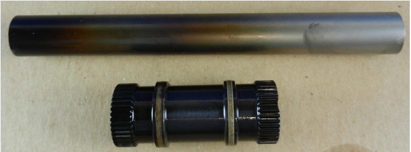
Turbine-To-Compressor Coupling and Power Turbine-To-Pinion Gear Coupling
