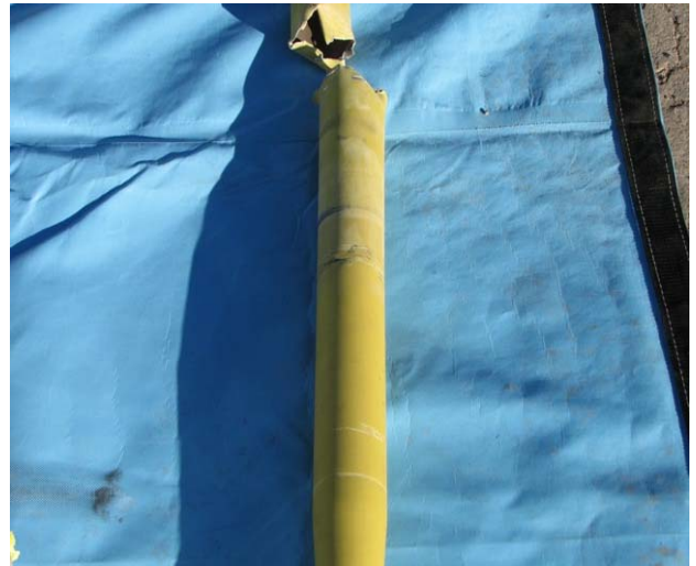
Tail rotor drive shaft scoring
