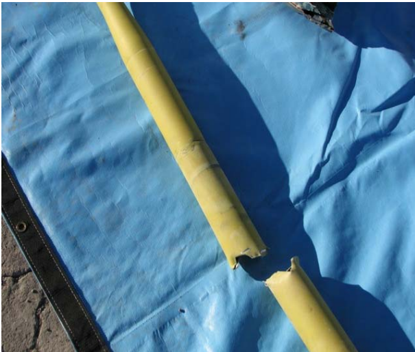
Tail rotor drive shaft separation
