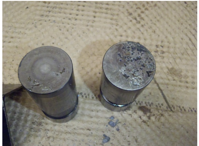
#6 lifters displaying spalling
