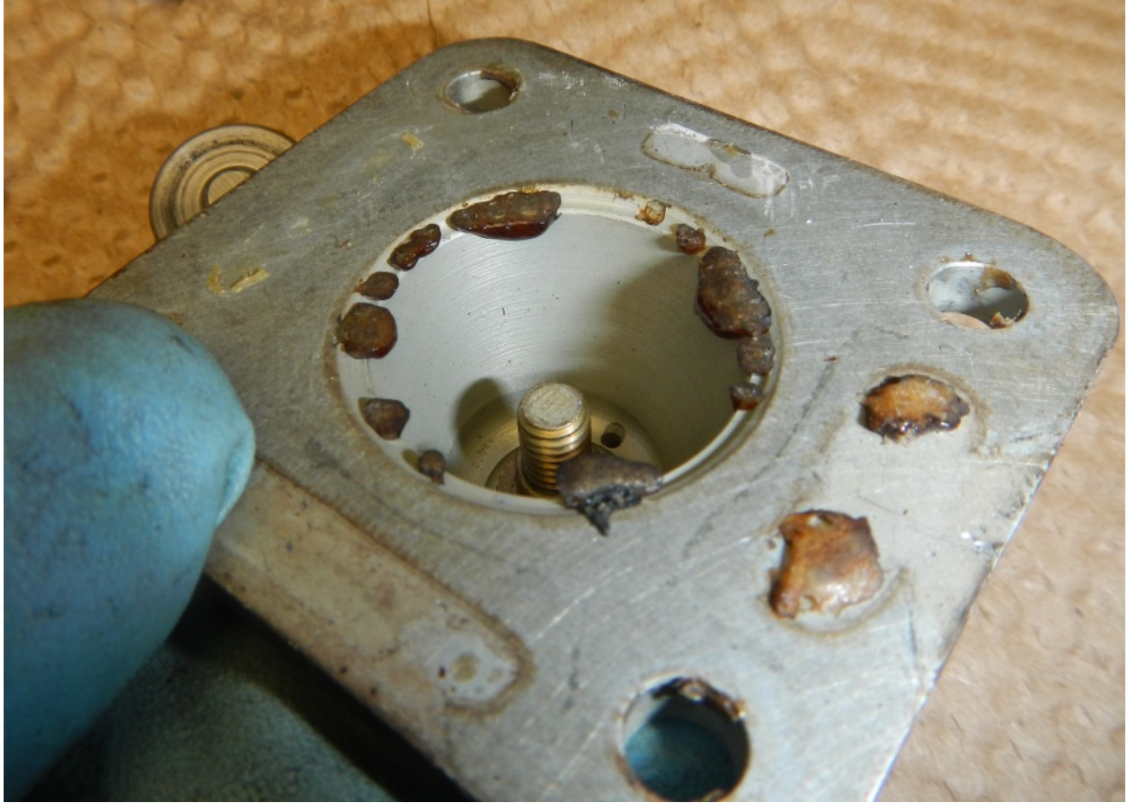
Figure 20 – Relief Valve Chamber with Gasket Thermal Deposits
