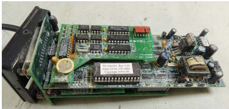
Figure 2. Damaged internal components of the JPI EDM-700.
