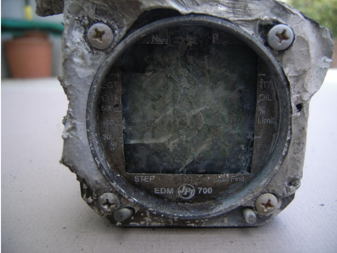
Figure 1. Fire damage to exterior of JPI device.
