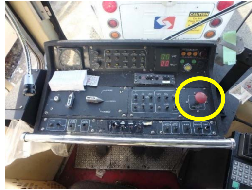
Figure 2. LRV operating console with the emergency brake push-button circled.
