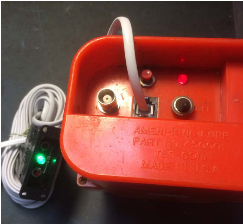
Figure 6 Lights Illuminated on Cockpit Remote Switch and Main Unit
