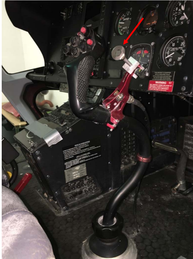
Figure 14. The red arrow points to the fixture installed on top of the activation handle.
