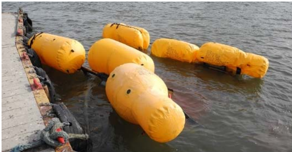
Figure 3. The six visible floats while the helicopter remained inverted in the East River.
