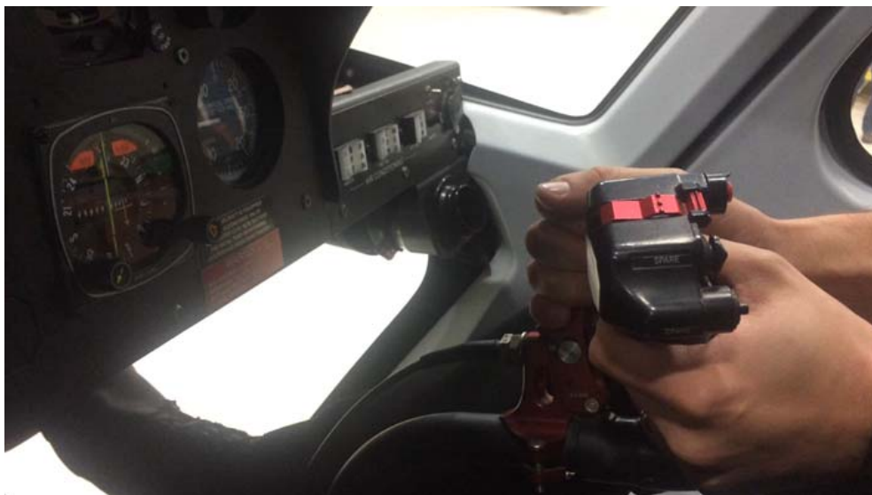
Figure 22. A screen-capture from the video for the emergency float system deployment as part of a 36-month inspection performed on December 14, 2016. The image shows the cyclic grip was braced with the left hand with the right hand on the emergency float system activation handle. (Video courtesy of Liberty Helicopters)
