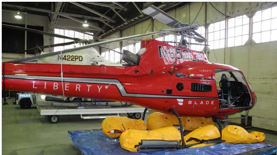
Figure 11. The three floats installed on the right skid.
