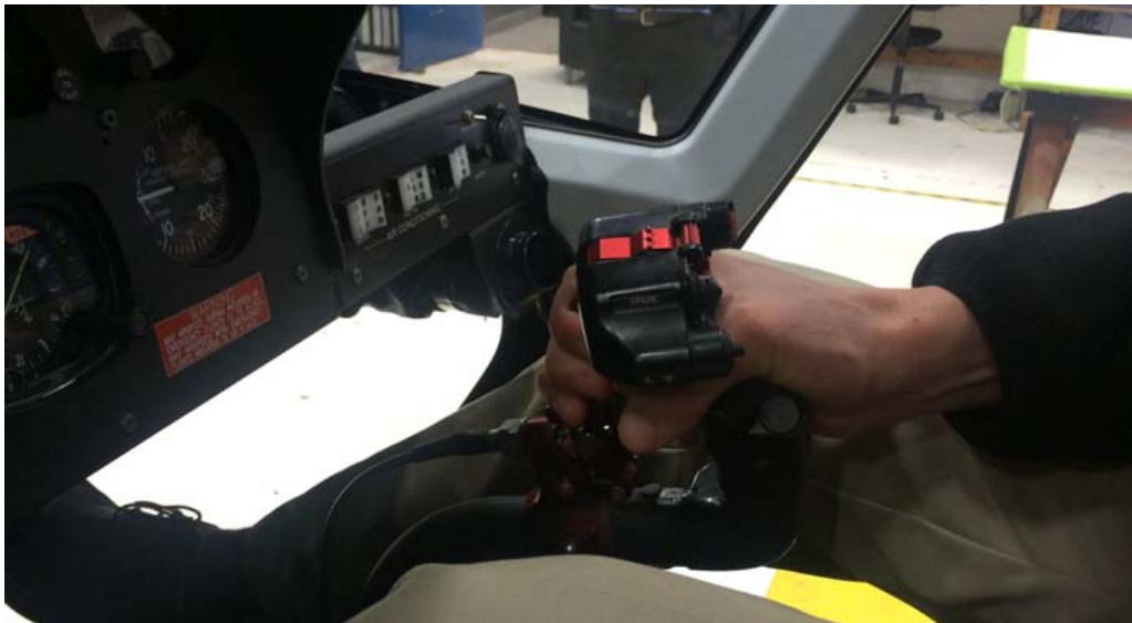
Figure 21. A screen-capture from a second video on March 1, 2017. The image shows the activation handle was in-line with the cyclic grip, resulting in contact with the cyclic head when the activation handle was pulled aft. (Video courtesy of Liberty Helicopters)
