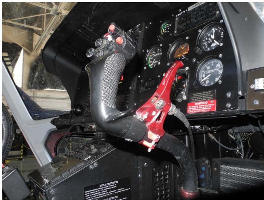
Figure 7. The activation handle installed on the cyclic control.
