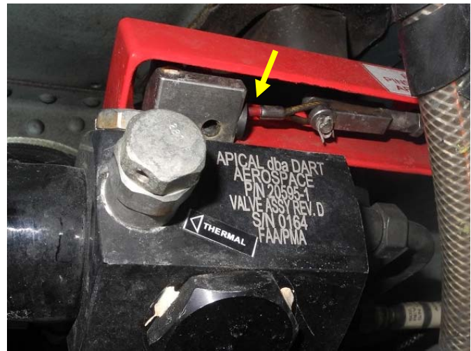
Figure 6. The right valve assembly. The yellow arrow points to the valve cable.
