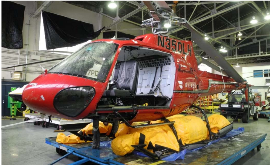
Figure 10. The three floats installed on the left skid.
