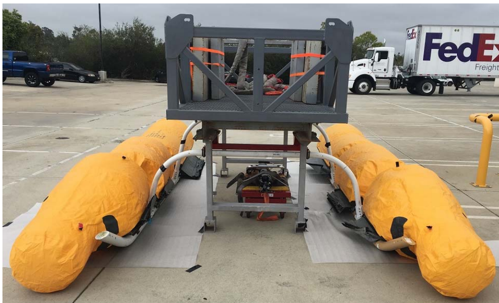
Figure 25. The inflated floats at the conclusion of the third inflation test.
