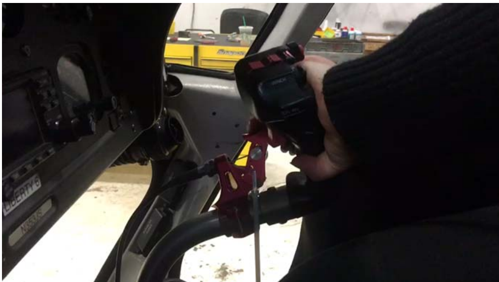
Figure 19. A screen-capture from the video for the emergency float system deployment as part of the 36-month inspection on N353JS. The image shows the cyclic grip was braced with the left hand while the right hand pulled aft on the emergency float system activation handle. (Video courtesy of Liberty Helicopters)
