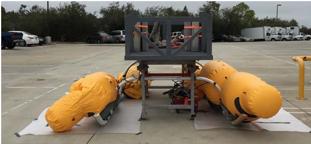
Figure 23. The inflated floats at the conclusion of the first inflation test.
