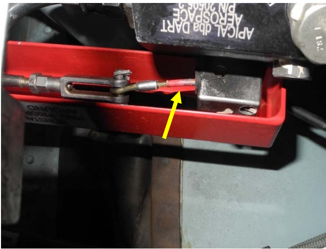
Figure 5. The left valve assembly. The yellow arrow points to the valve cable.
