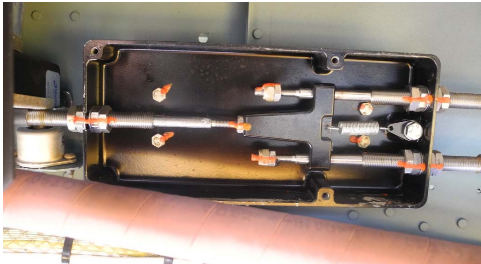
Figure 9. A view of the junction box showing the gap of about 0.75 inches between the cable nuts and the dual cable block after a continuity check was performed by pulling the activation handle. Prior to the continuity check, the pull cables were disconnected at the left and right valves.
