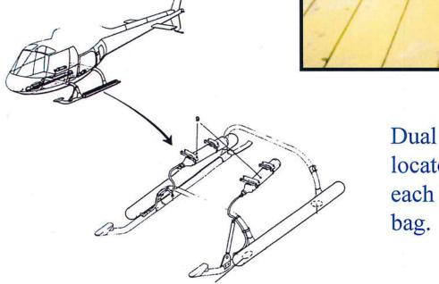
Dual pressurized helium bottles located under aft belly panel, each bottle supplies its own float bag.
