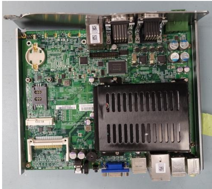
Figure 12. The PSC data logger with the external casing removed.
