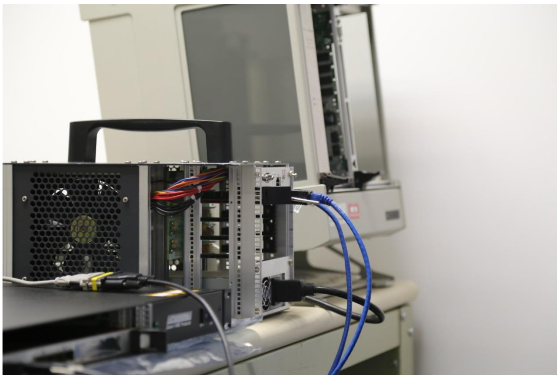
Figure 11. Power applied to the test card with the accident board installed.
