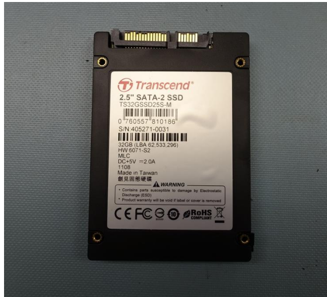
Figure 13. The PSC data logger's solid state drive in the condition it was extracted from the device.
