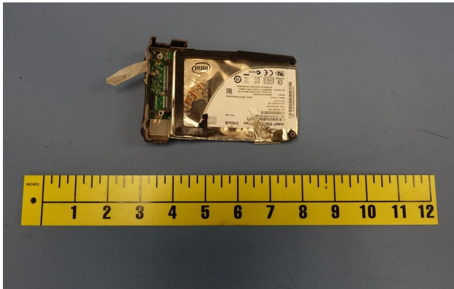
Figure 5. The "SS AFT CAM" Hard Drive as Recovered from the SS2 Wreckage.
