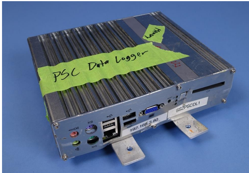
Figure 2. The pressurization system controller data logger.
