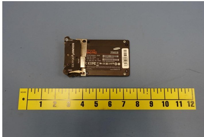
Figure 6. The “SS Boom Cam” Hard Drive and the Associated PIX Chassis Connector.
