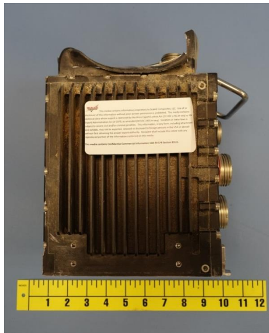
Figure 1. The RMC as recovered from wreckage site # 2 1 .
