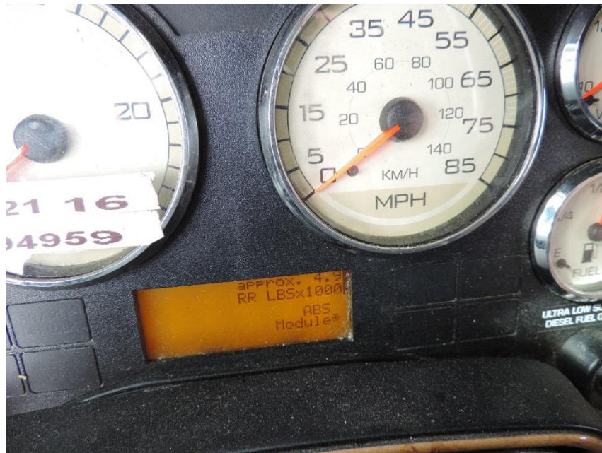
Figure 14. RR thousand pounds of the tractor trailer displayed on the instrument panel. The screen read approx. 4.9 thousand pounds.
