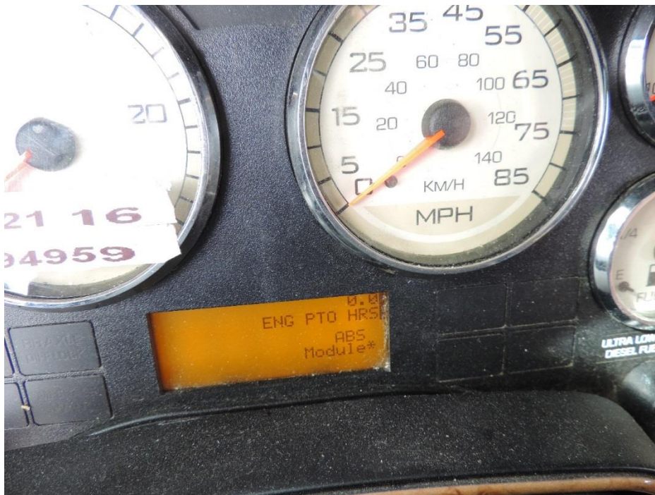
Figure 9. Total Engine PTO hours of the tractor trailer displayed on the instrument panel. The screen read 0.0 hours.
