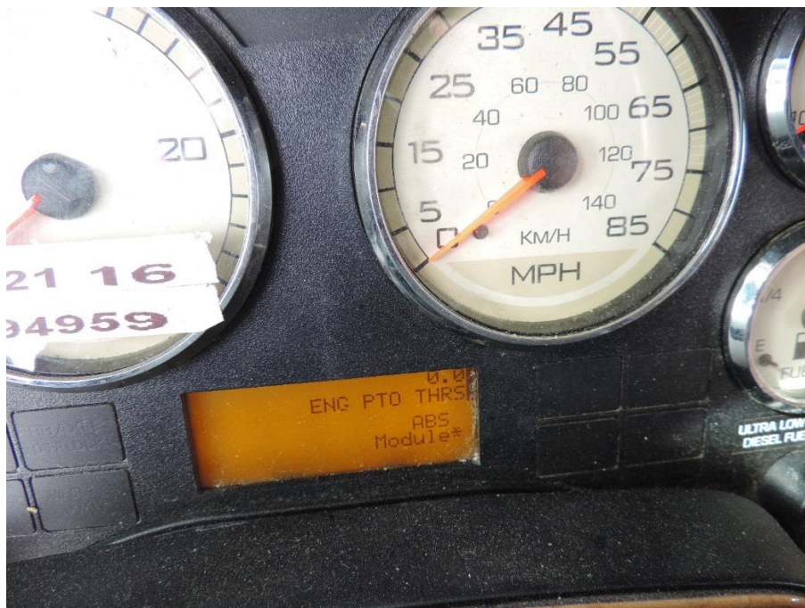
Figure 9. Total Engine PTO hours of the tractor trailer displayed on the instrument panel. The screen read 0.0 hours.
