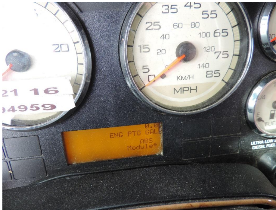
Figure 13. ENPTO TR gallons of the tractor trailer displayed on the instrument panel. The screen read 0.0 gallons.
