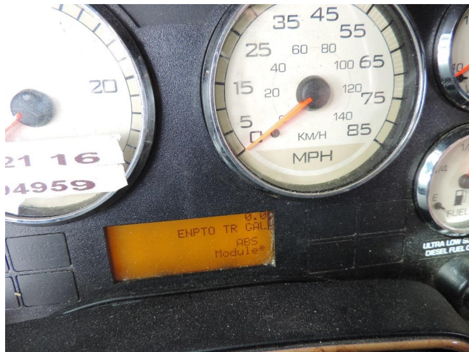
Figure 13. ENPTO TR gallons of the tractor trailer displayed on the instrument panel. The screen read 0.0 gallons.
