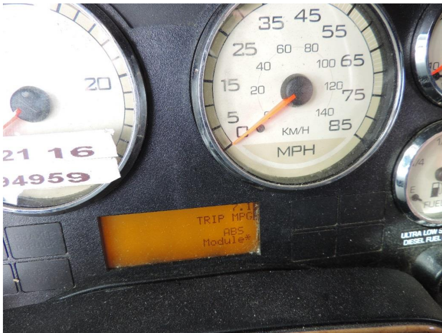
Figure 11. Trip miles per gallon (MPG) of the tractor trailer displayed on the instrument panel. The screen read 7.1 mpg.
