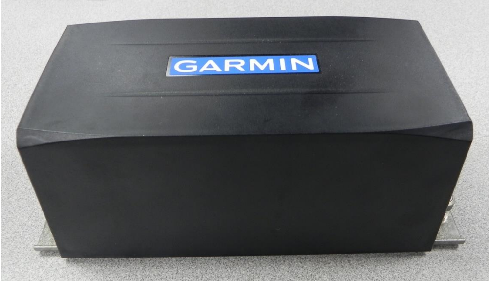
Figure 3. External view of the Garmin GRS-77 attitude heading and reference system (AHRS).
