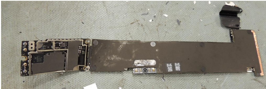
Figure 4. Apple iPad 2 main circuit board removed.
