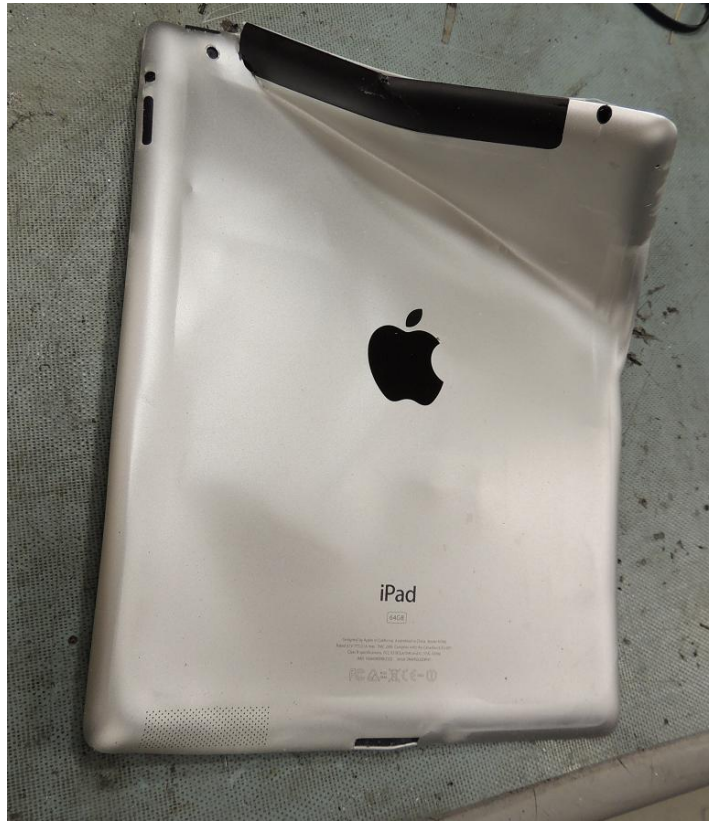
Figure 2. Apple iPad 2 damage – back.
