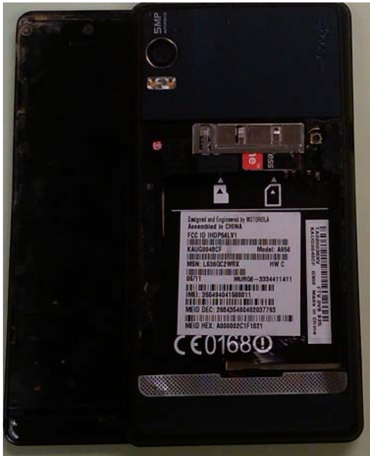
Figure 5. Back of Droid showing minor damage and missing battery.
