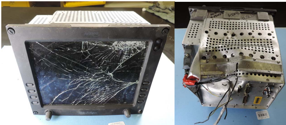
Figure 2. Front and back of the Avidyne PFD as received.
