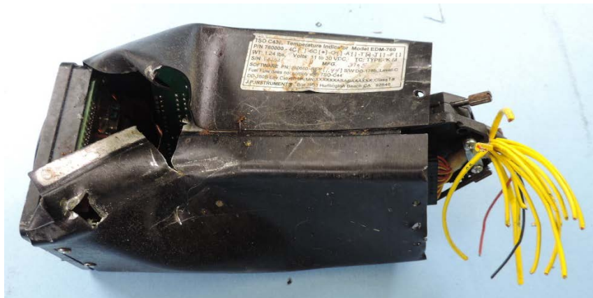
Figure 1. JPI EDM-760 as received.
