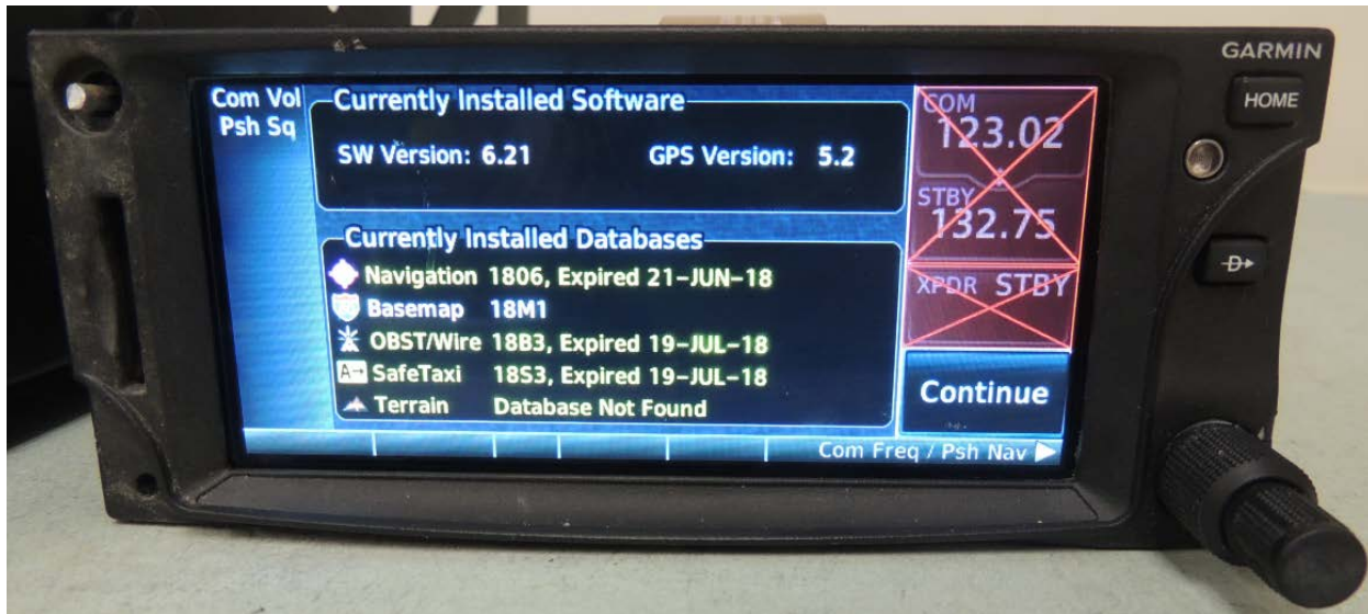
Figure 3. Garmin GTN 650-866 firmware and last frequency
