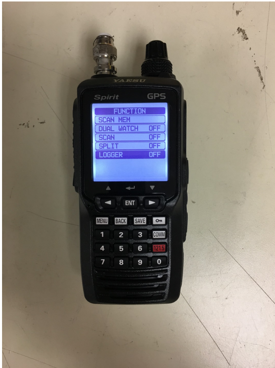
Figure 3. Yaesu Spirit GPS menu showing showing "Logger" function set to "OFF"
