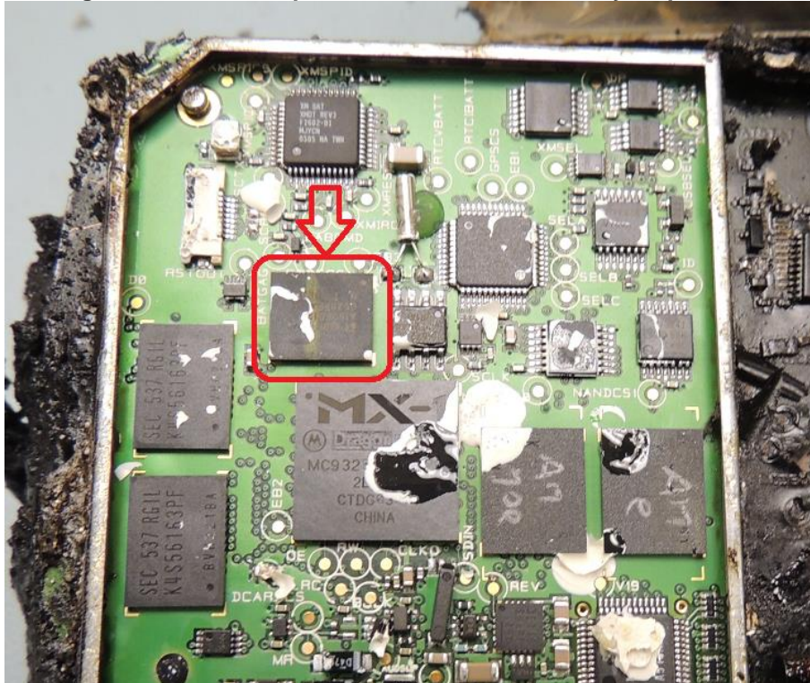
Figure 3. Internal inspection; non-volatile memory chip annotated.
