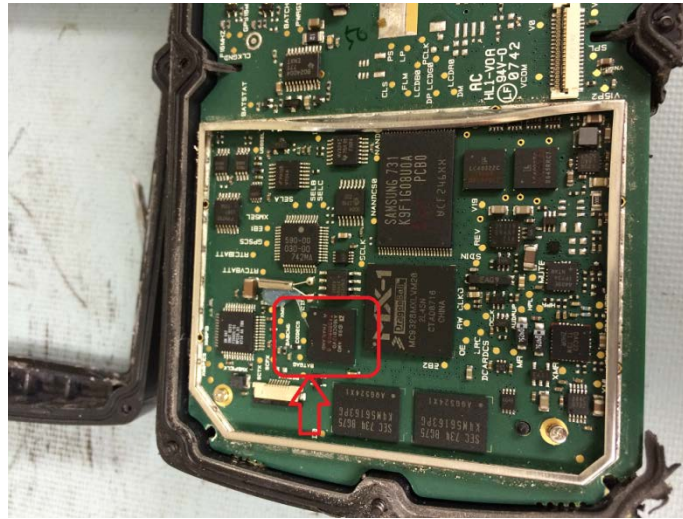
Figure 2. Garmin GPSMAP 396 internal, with non-volatile memory annotated.
