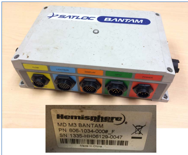
Figure 1. Photo of Satloc M3 and dataplate.
