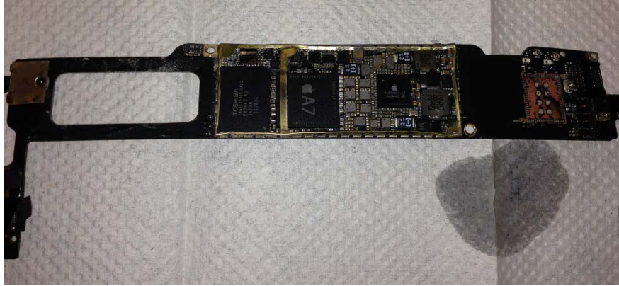
Figure 2. Internal board removed and cleaned.
