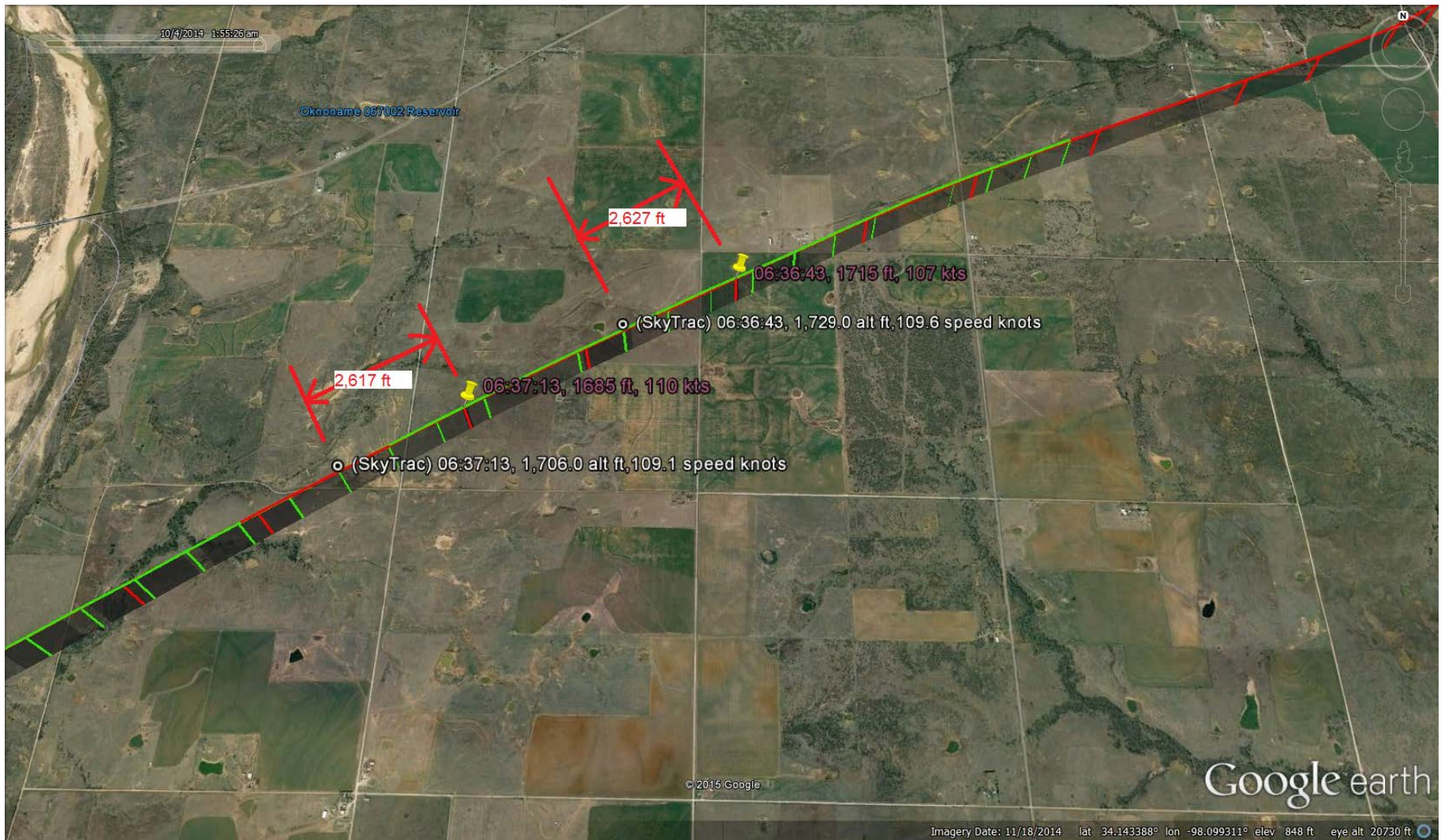
Figure 19. Comparison of Garmin GPSMAP 396 and SkyTrac ISAT-100, enroute.
