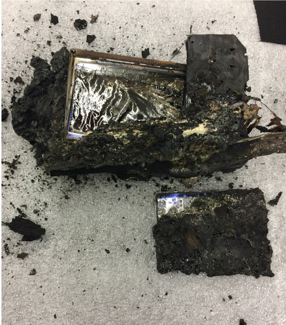
Figure 2. Partially intact Garmin GPSMAP 396.
