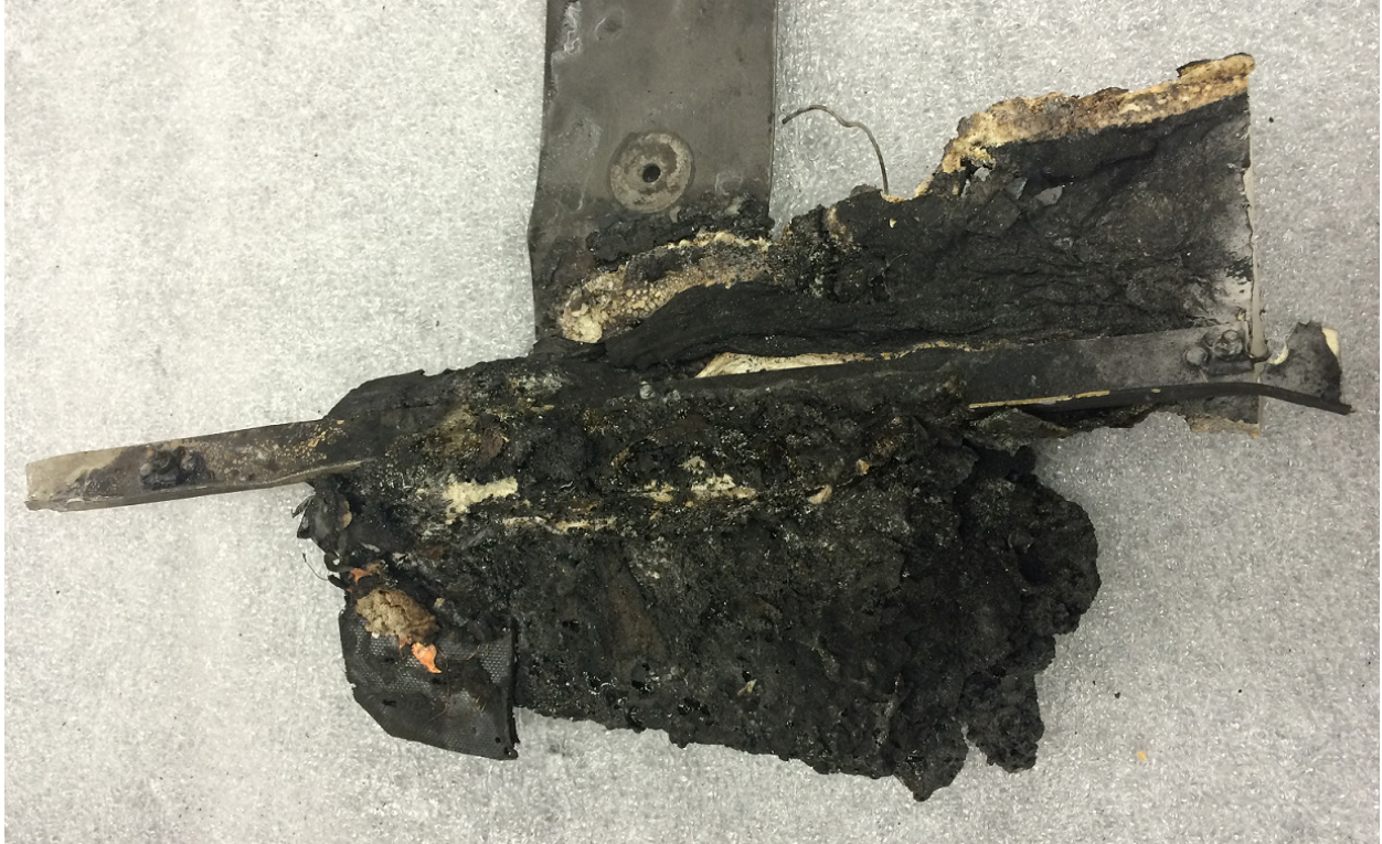
Figure 1. Charred encasement containing Garmin GPSMAP 396.
