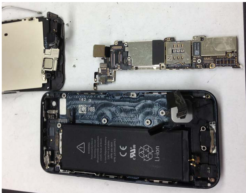
Figure 7. Apple iPhone 5 disassembled.
