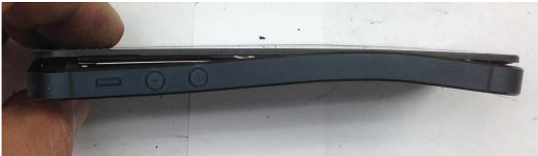
Figure 6. Apple iPhone 5 impact damage.
