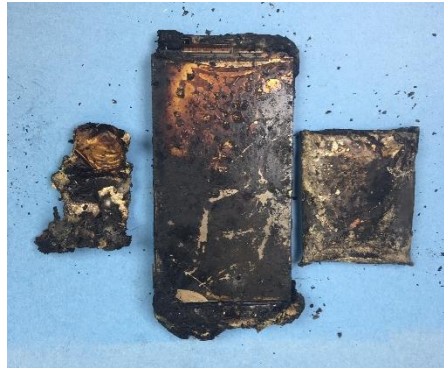
Figure 10. The rear of the unknown Android type PED and the device's battery.
