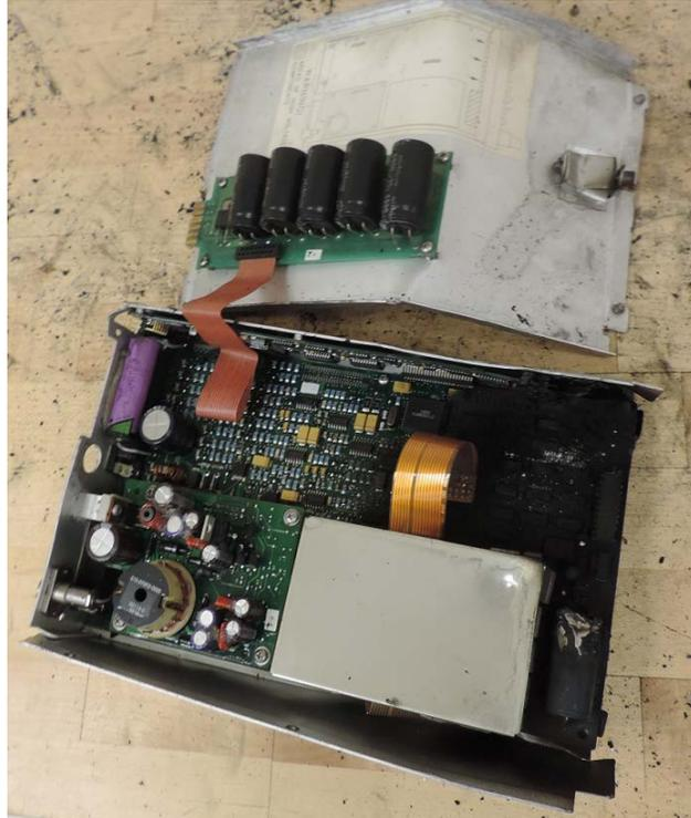
Figure 3 shows the Garmin 430W as received, and figure 4 shows the internal components of the device. The database cards were missing from the device. The Garmin 430W does not record track history and retains few state parameters (for example, last frequencies). Given the damage, no recovery was attempted.
