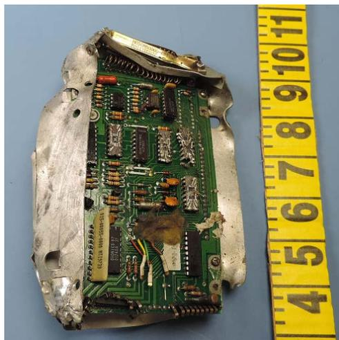
Figure 9 shows a printed circuit board (PCB), as received. Exterior inspection was insufficient to determine the origin of the PCB. The non-volatile memory chips were
