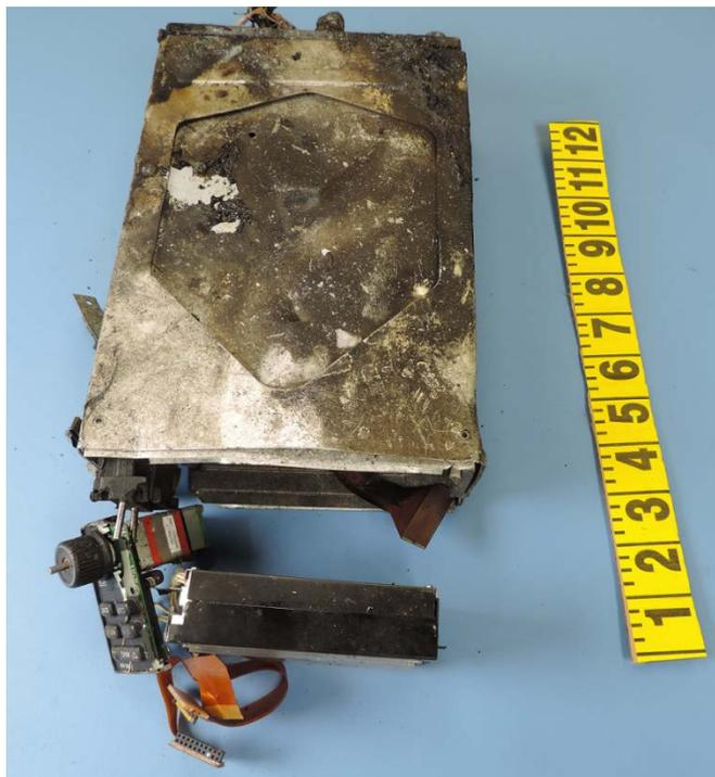
**Figure 4. Device 2: Garmin 430W, internals.**
