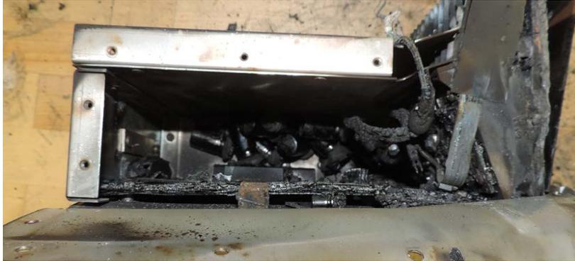
Figure 7 shows the Trans Cal Altitude Digitizer. According to the manufacturer, the device did not record any historical data; thus, no data recovery was attempted.
