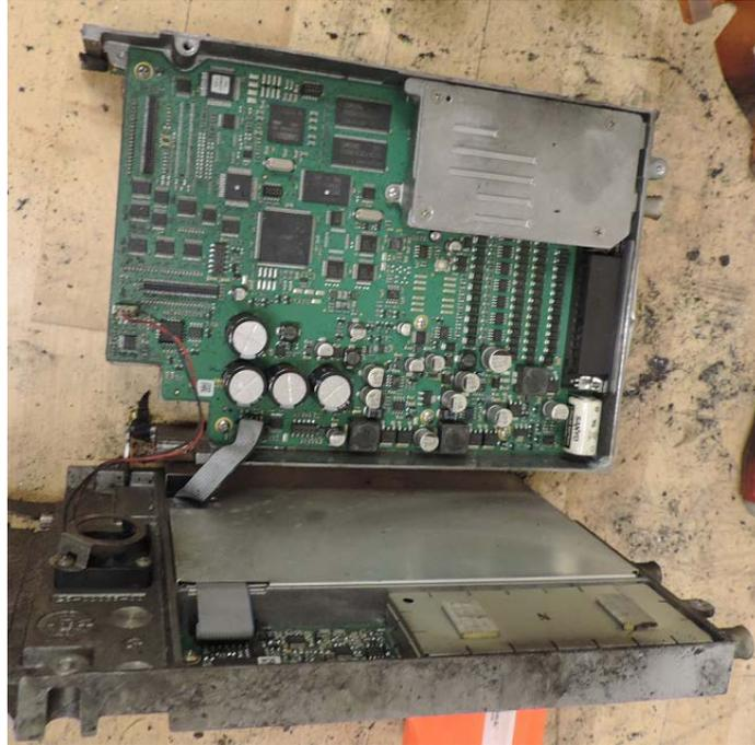
Figure 5 shows the Garmin GMX200, with its exterior mounting rack removed. Figure 6 shows the internal inspection, with most electronic components destroyed by heat damage. No recovery was possible due to the heat damage.
