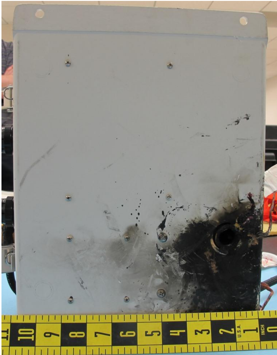
Figure 4 - Bottom of Power Distribution Box
