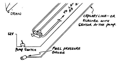
The accompanying sketch outlines the fuel system. It is a two-tank, selectable, pumped (not gravity) system with an engine-driven pumpplus an electrical backup pump. This is similar to most low-wing light planes -Grummon, Piper and Beech.
