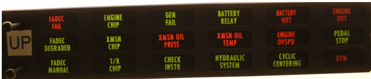
Caution Advisory Panel – Right Side
