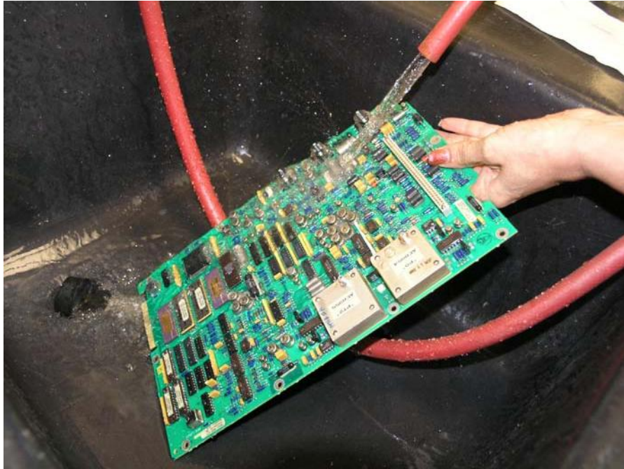
Figure 13. 45-CF0149 DEEC Circuit Card Being Rinsed with De-Ionized Fresh Water
