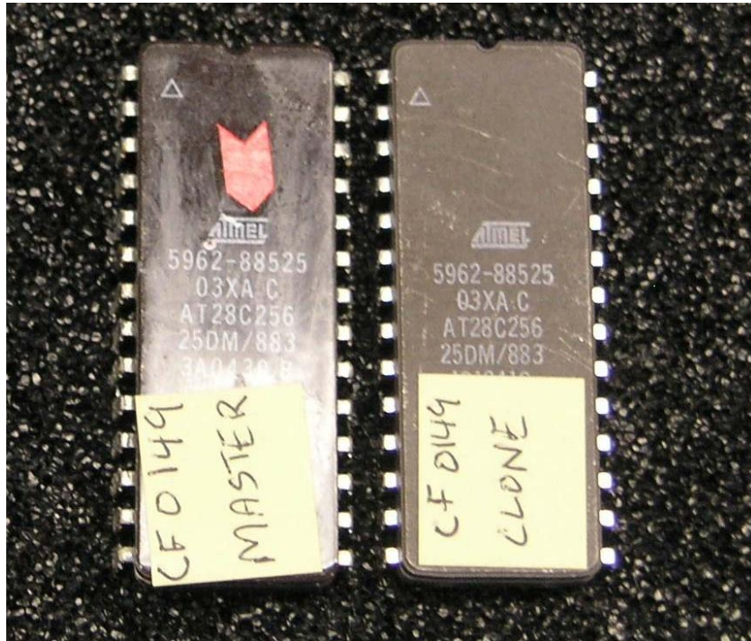
Figure 39. NVM Chip Data CF0149 Copied to a Clone IC
