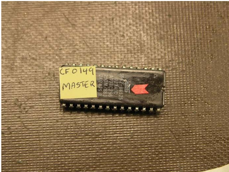
Figure 36. CF0149 NVM Chip Labeled After Removal From Circuit Card
