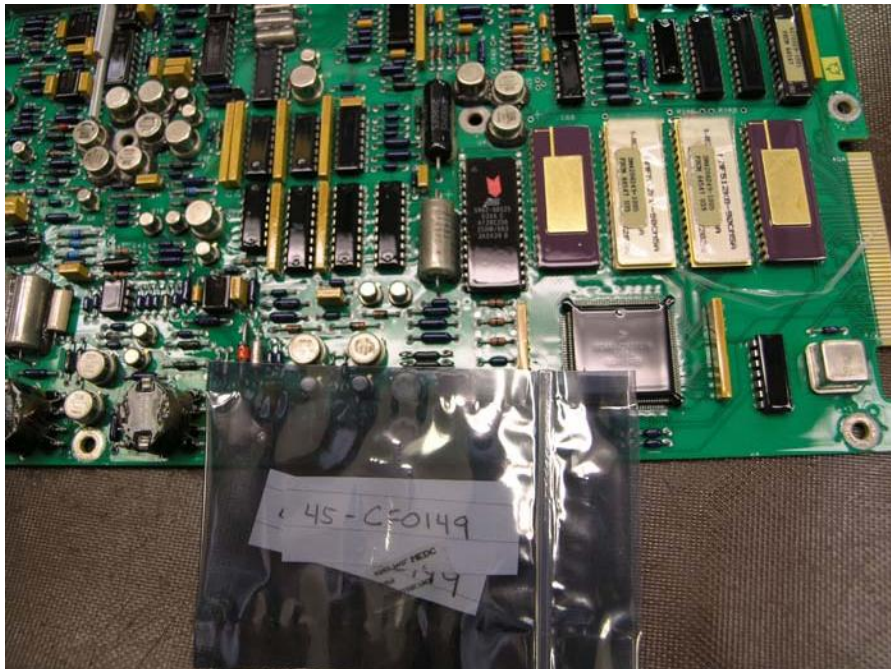
Figure 34. CF0149 (Left Engine) N1 DEEC Circuit Card and NVM Chip
