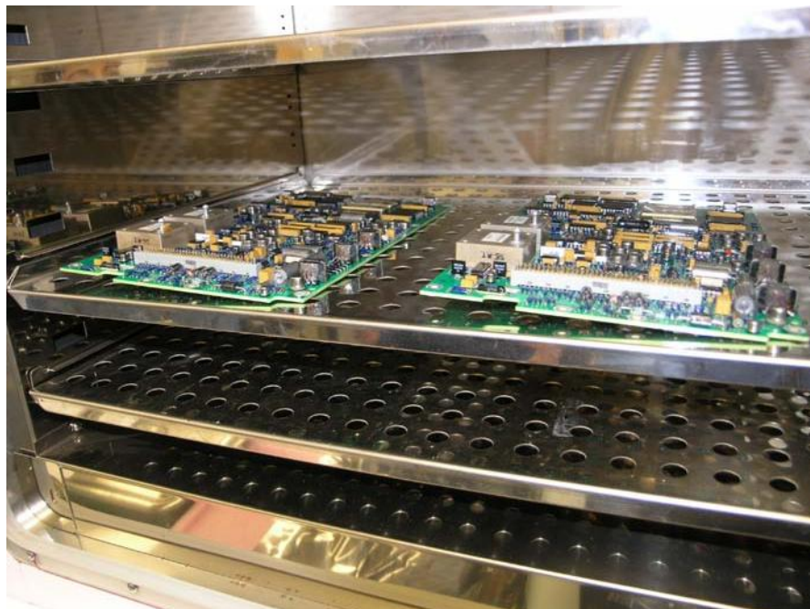
Figure 16. DEEC Circuit Cards in Drying Oven
