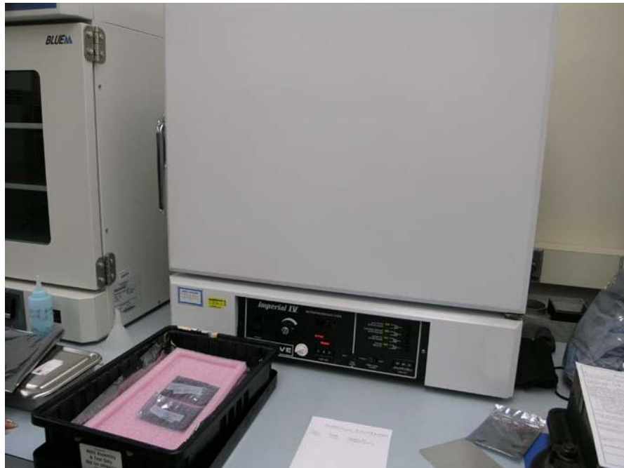
Figure 18. Oven Used for Drying DEEC Circuit Cards
