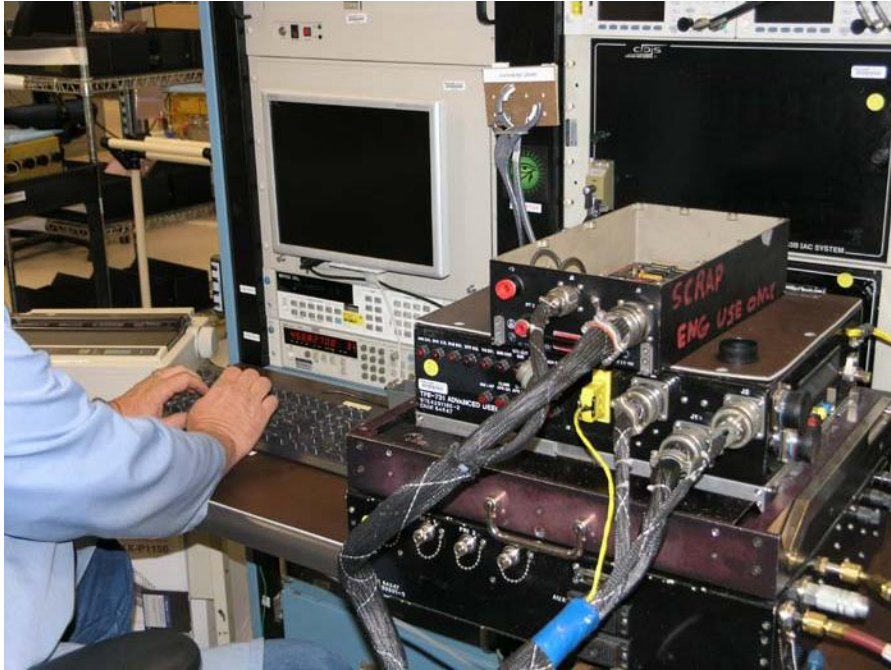
Figure 41. Slave N1 DEEC Being Downloaded
