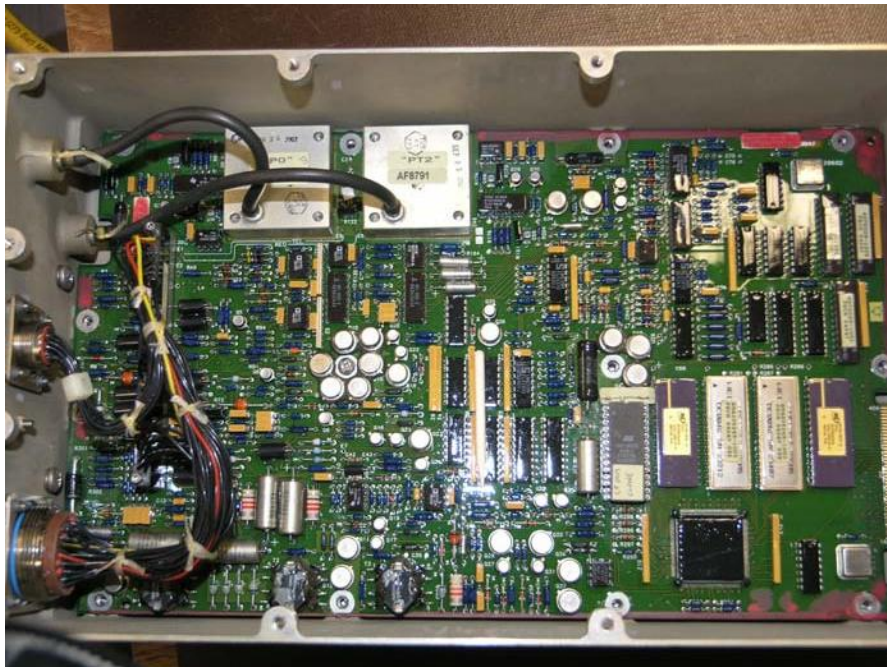
Figure 40. CF0149 Clone NVM Chip Installed into Slave N1 DEEC
