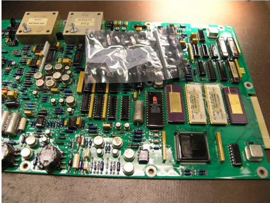
Figure 43. CF0152 (Right Engine) N1 DEEC Circuit Card and NVM Chip
