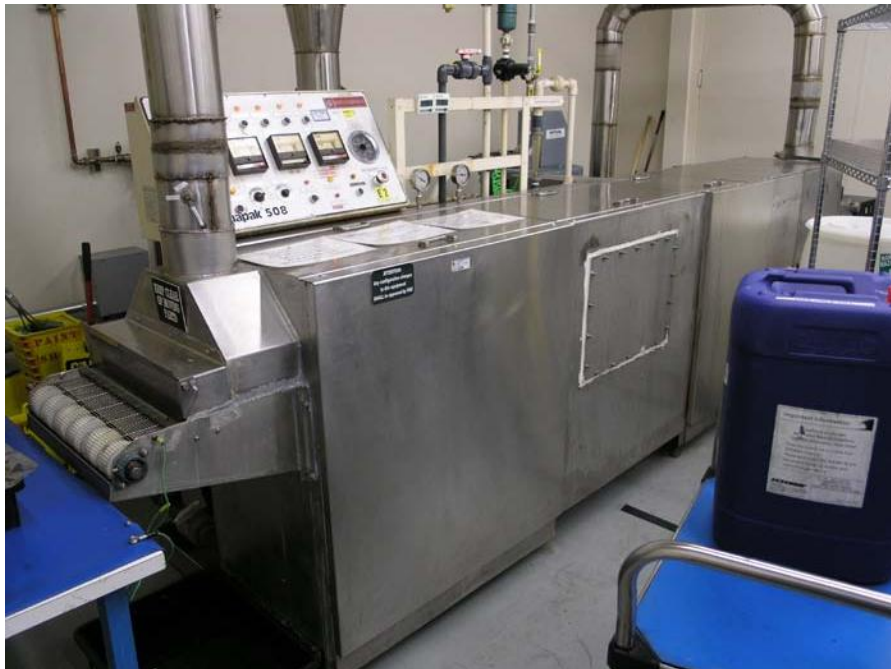
Figure 14. 45-CF0149 DEEC Circuit Card Undergoing Zestron Cleaning Process
