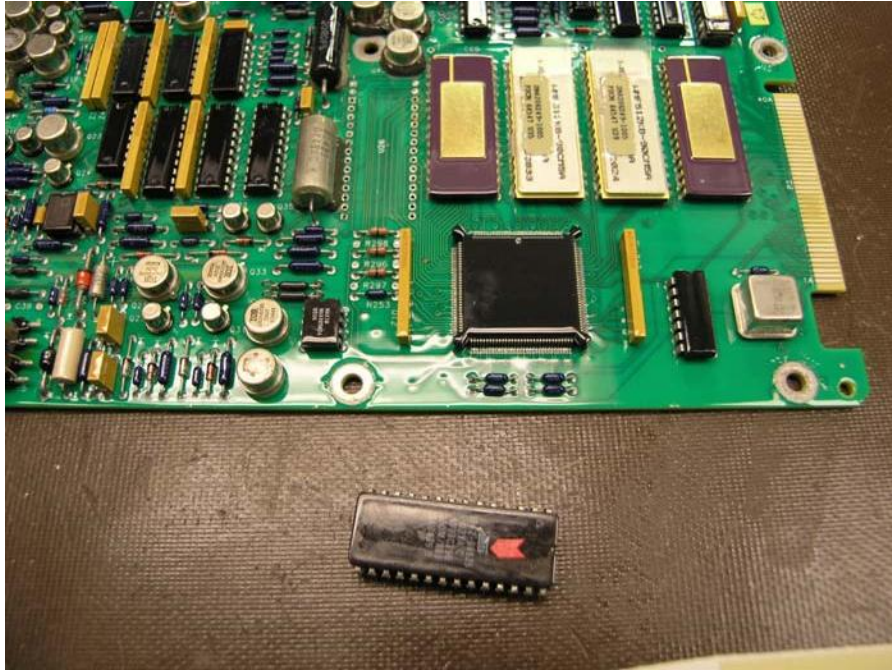
Figure 35. CF0149 (Left Engine) N1 DEEC NVM Chip After Removal
