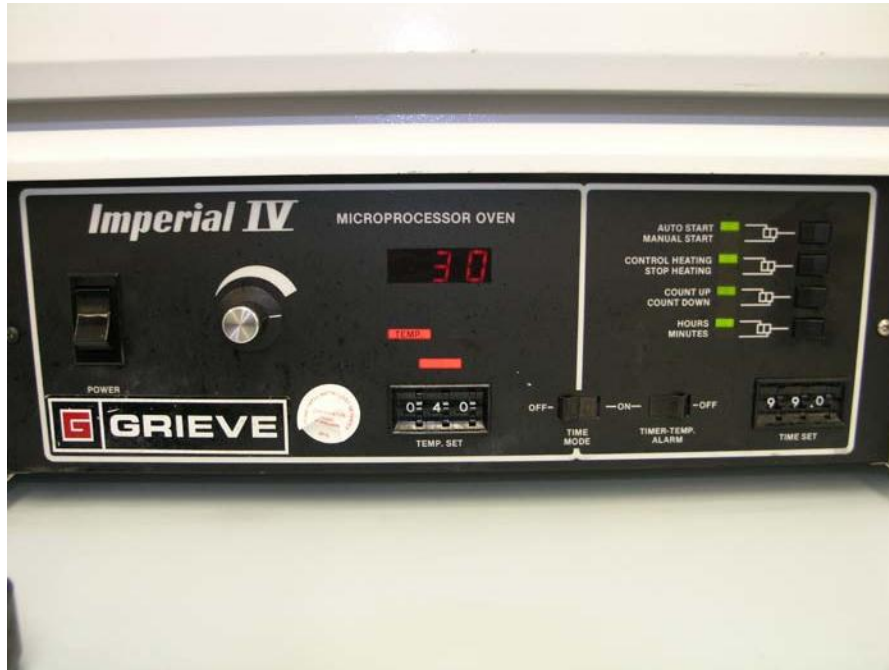
Figure 17. Oven Used for Drying DEEC Circuit Cards
