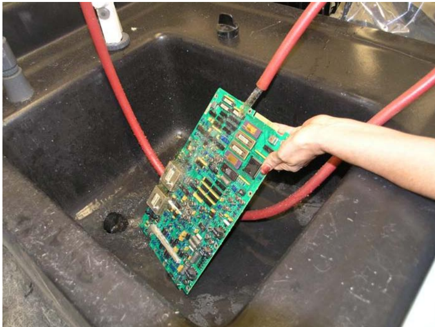
Figure 30. 45-CF0152 DEEC Circuit Card Being Rinsed with De-ionized Fresh Water
