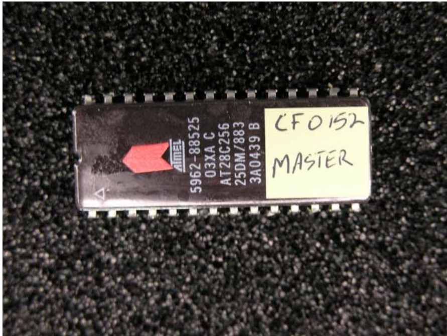
Figure 45. CF0152 NVM Chip Labeled After Removal From Circuit Card
