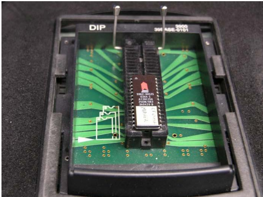
Figure 46. CF0152 MASTER NVM Chip Installed in Data IO Programmer
