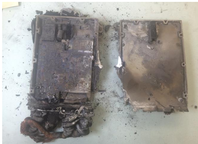
Figure 2. The DECU after its external housing was carefully opened with a cutoff wheel.
