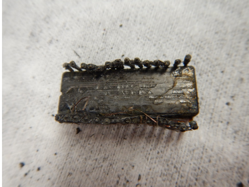
Photo No. 6: Underside of chip also showing the bent pins.(Honeywell)
