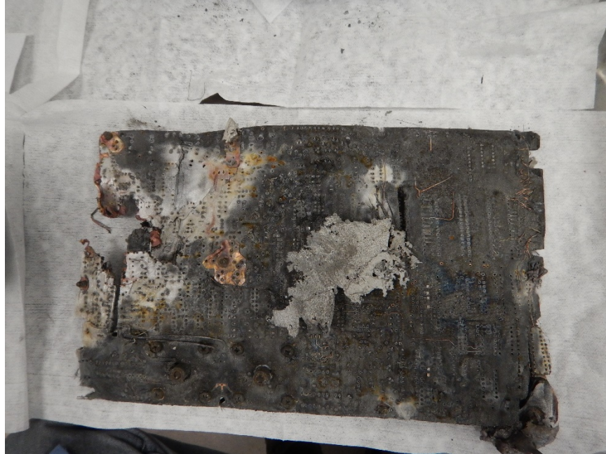
Photo No. 4: Underside of board "A" showing metal slag. (Honeywell)
