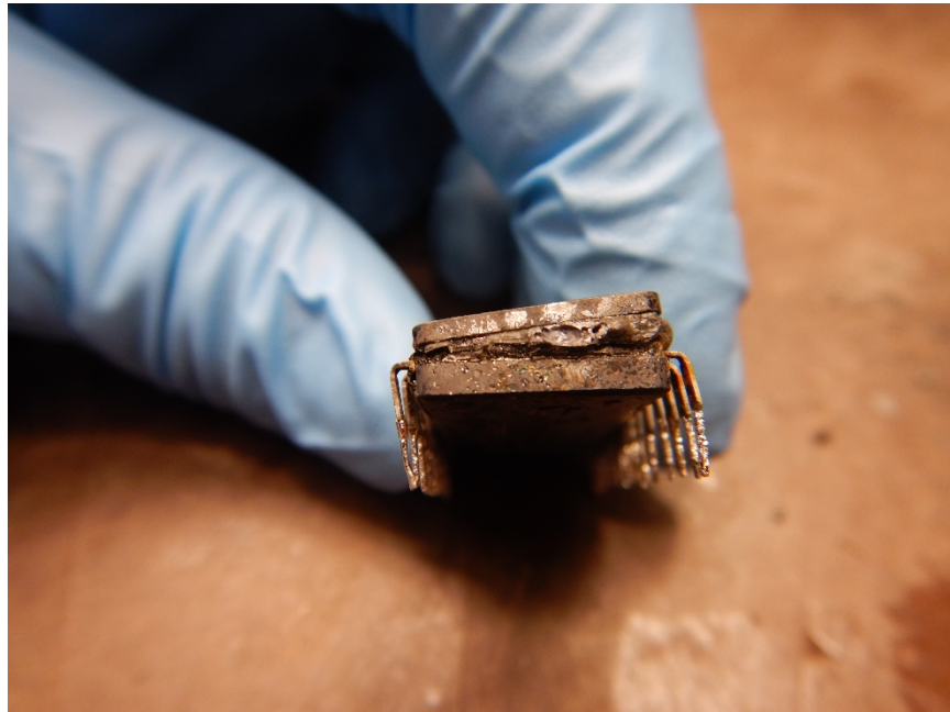
Photo No. 7: Side view of chip showing partially lifted cover. (Honeywell)
