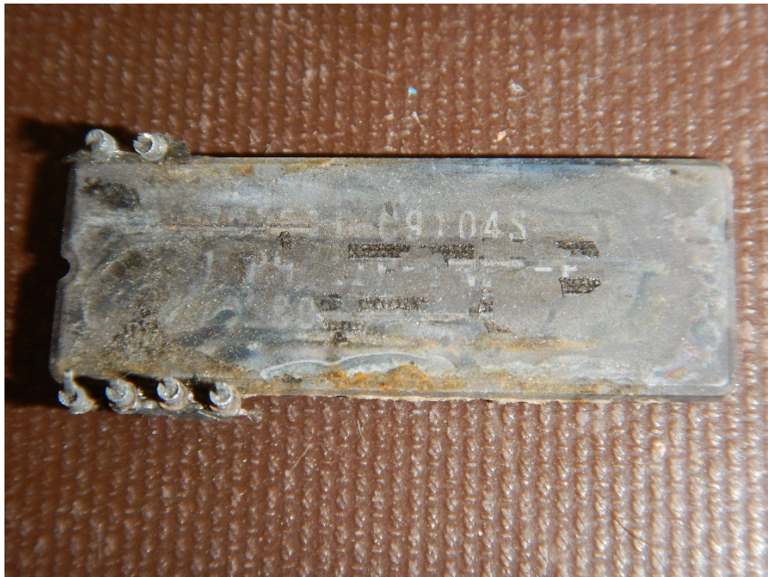
Photo No. 14: Markings on underside of memory chip from accident DEEC. (Honeywell)
