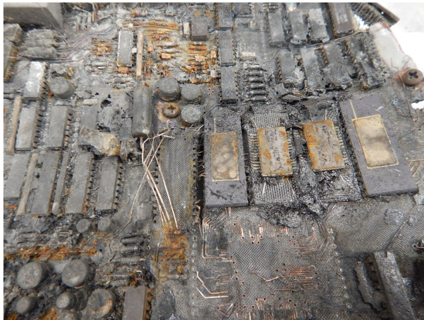
Photo No. 3: Close up view of board "A" showing exposed fiberglass matting. (Honeywell)
