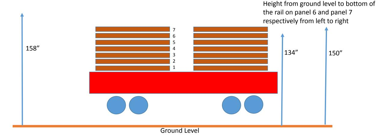
Width of panel - tie end to farthest base of rail 78" 11,200 lbs is weight of panel, indicated by stencil
