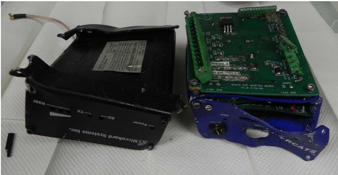
Figure 6 - DCU, sensor adaptor and RF transmitter
