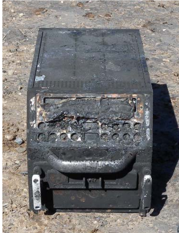
Figure 7 – Solid state data cartridge removed from Heim flight recorder.
