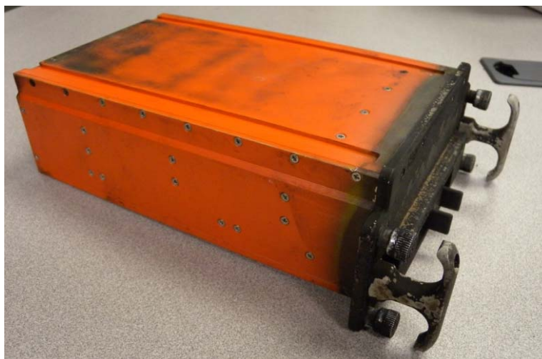
Figure 7 – Solid state data cartridge removed from Heim flight recorder.
