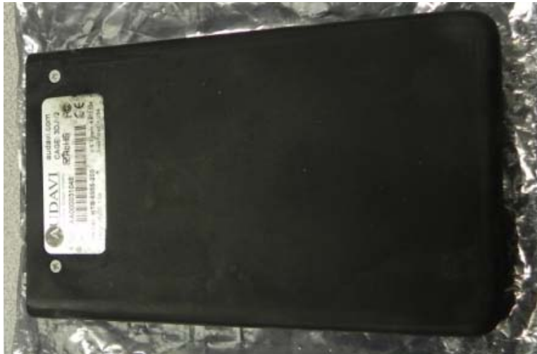
Figure 8 – An example of a removable hard disk drive from the IADS server.
