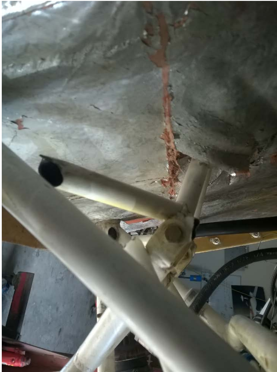
Photo 1 – View of firewall damage (photo courtesy of the pilot).
