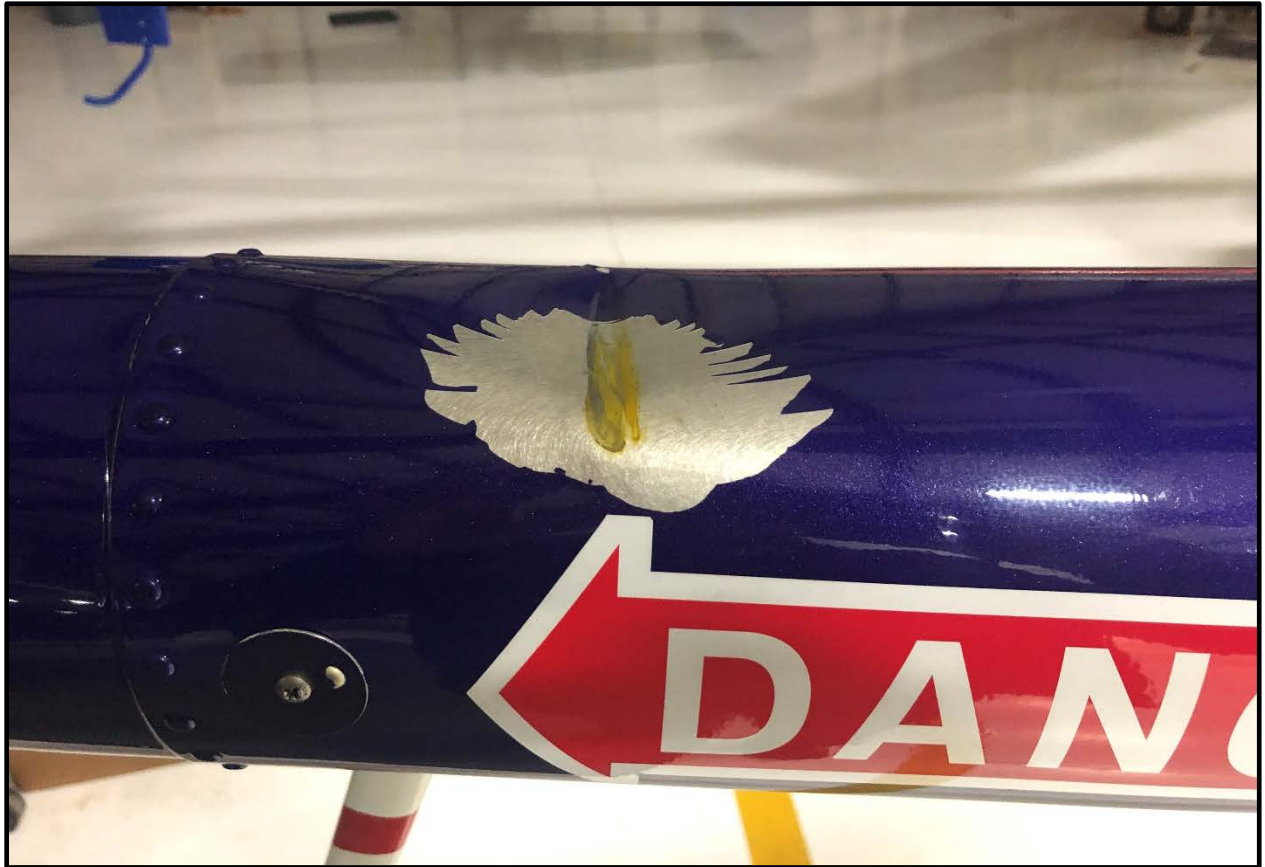
Figure 1: Dent in the tail boom.
