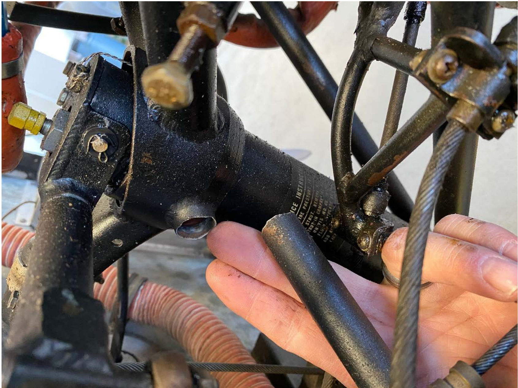
Photo 2 - View of engine mount damage (photo courtesy of photo courtesy of Velocity Air Inc.)
