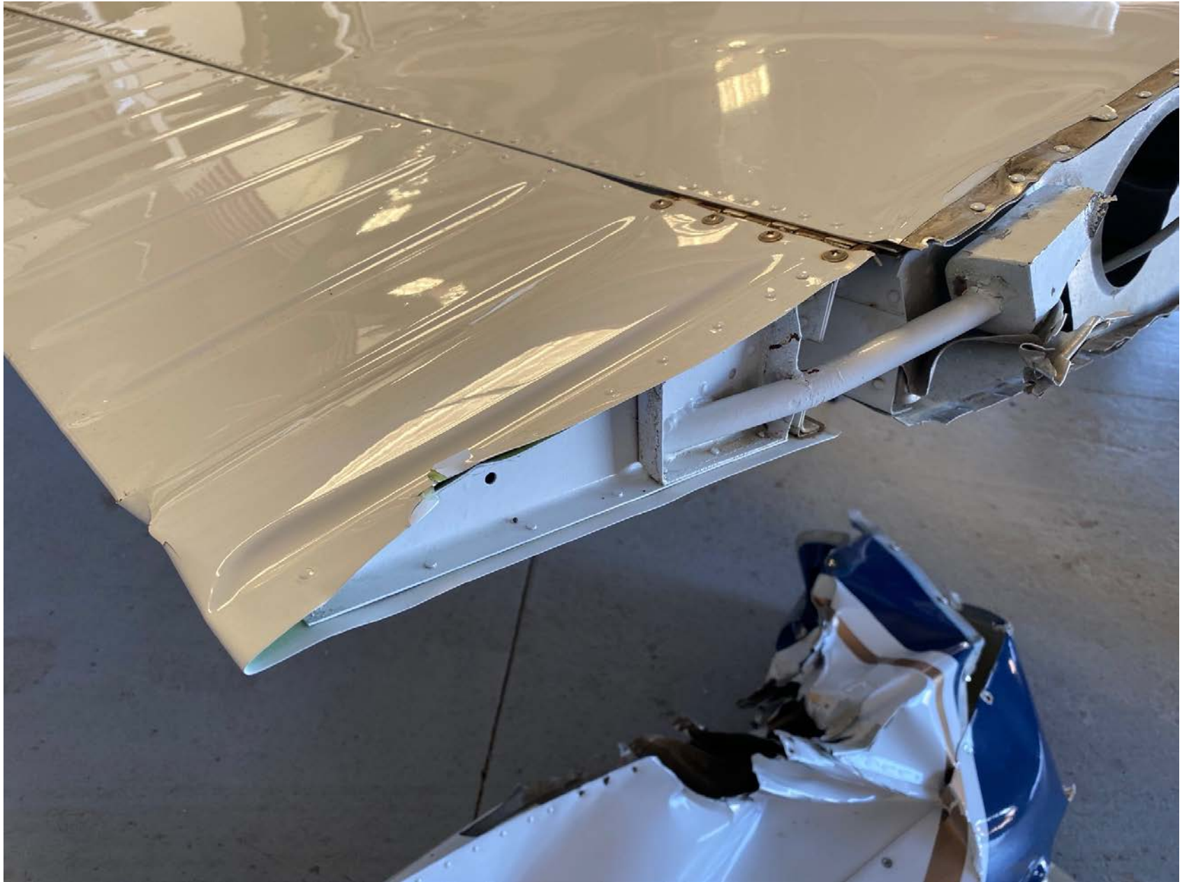
Photo 1 – View of right wing damage (photo courtesy of Velocity Air Inc.)
