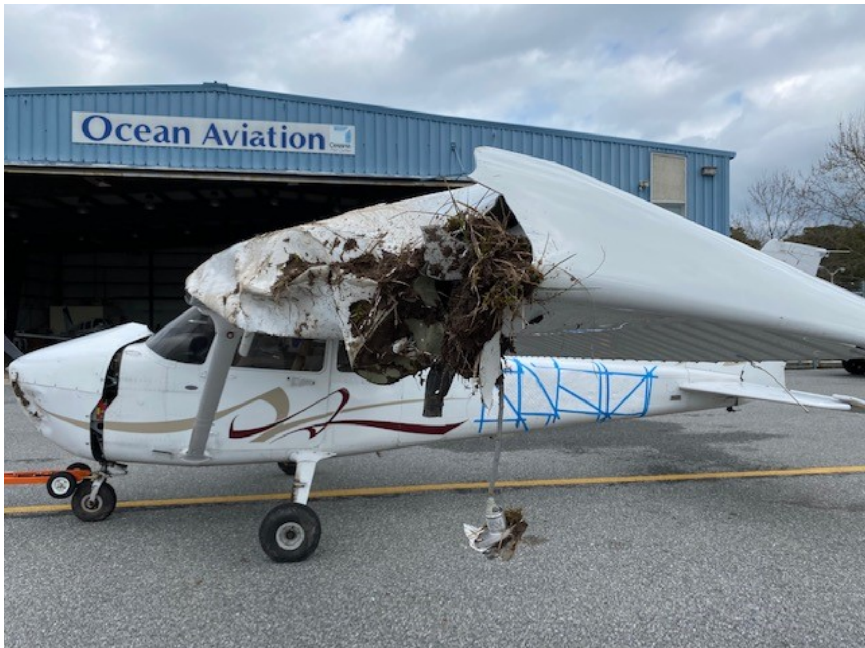
Photo 1 – View of left wing damage (photo courtesy of the operator)
