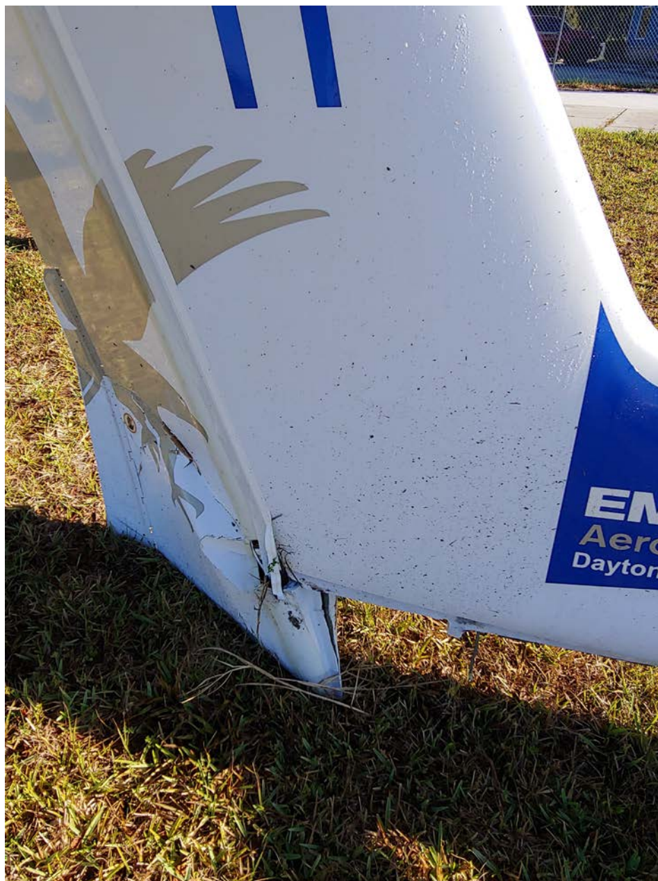
Photo 1 – View of rudder damage (photo courtesy of the FAA)
