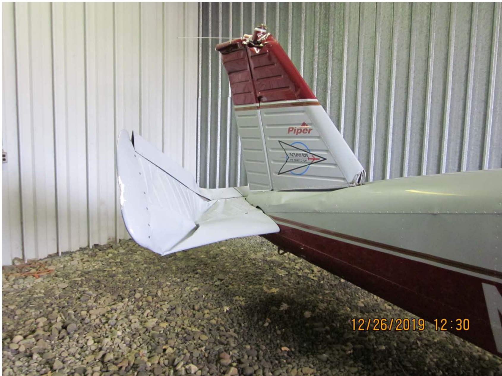
Photo 2 - View of empennage damage (photo courtesy of the FAA)
