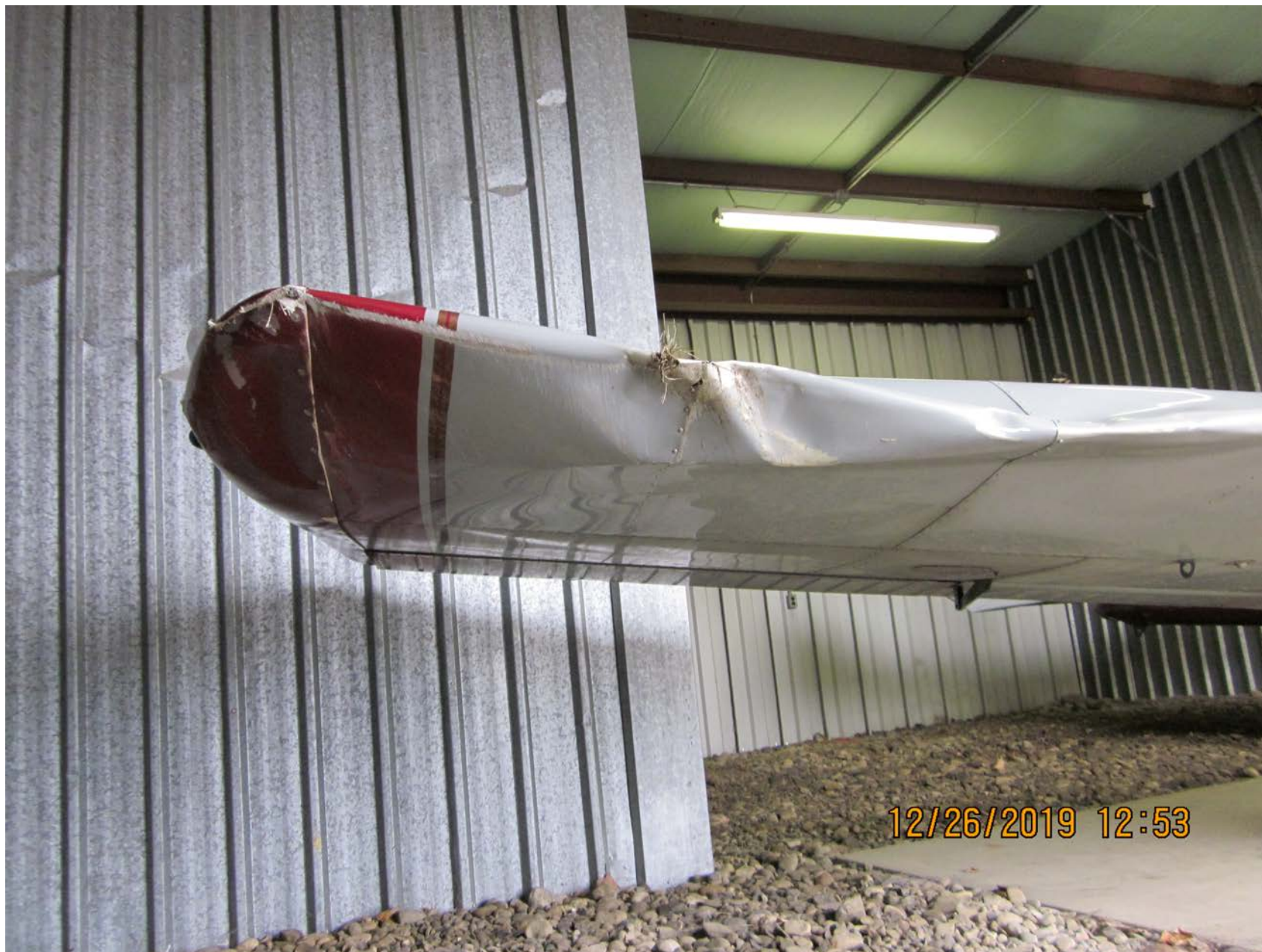
Photo 3 - View of right wing damage (photo courtesy of the FAA)
